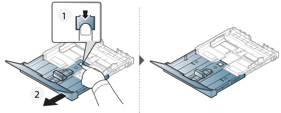
For paper smaller than Letter-sized, press and unlatch the guide lock in the tray, push the tray in manually. Then adjust the paper length guide and paper width guide.
