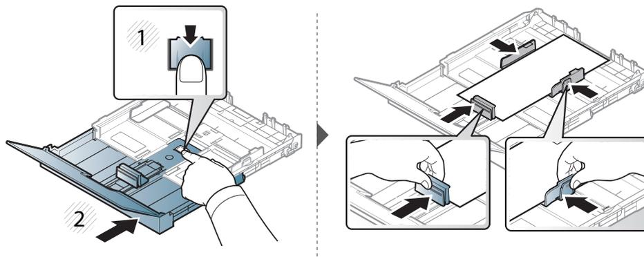
For paper longer than Legal-sized, press and unlatch the guide lock in the tray, pull the tray out manually. Then adjust the paper length guide and paper width guide.
