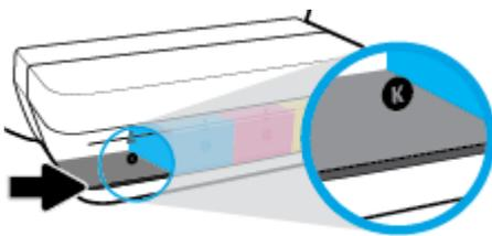
When you refill the ink tanks, fill the ink to the maximum lines only. Any ink level above the maximum line may cause ink leakage.
