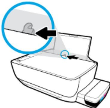
3. Insert a stack of small-size paper (like photo paper) into the far-right side of the input tray with the short edge down and the print side up, and slide the stack of paper down until it stops.
