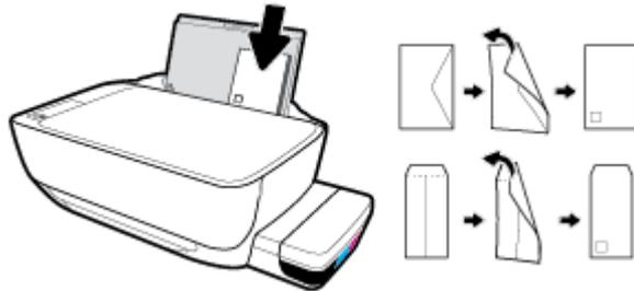
4. Slide the paper-width guide to the right against the stack of envelopes until it stops.
