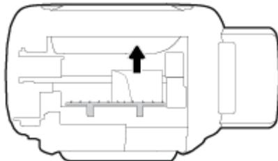
5. Close the cleanout door. Gently push the door towards the printer until both latches snap into place.
