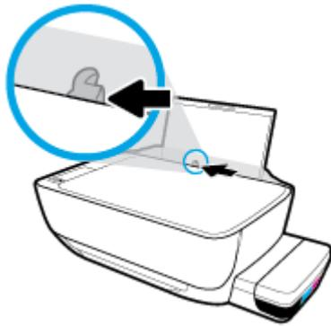
3. Insert one or more envelopes into the far-right side of the input tray and slide the stack of envelopes down until it stops.
