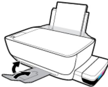
3. Remove and reinsert the printhead.
