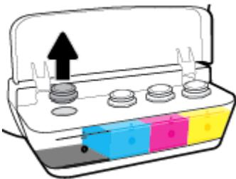
3. Twist to remove the cap of the ink bottle, remove the seal from the bottle, install the cap back onto the bottle, and then pull open the top part of the cap.
