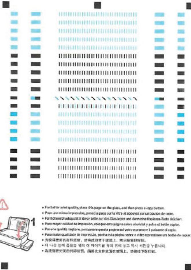
5. Follow the onscreen instructions to load the printhead alignment page print side down on the scanner glass, and then click **Scan** to scan the alignment page.
