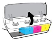
2. Remove the cap of the ink tank you plan to refill.
