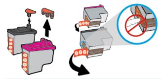
NOTE: Do not touch the electrical contacts on the printhead.
