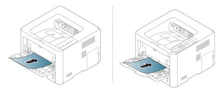
3 Squeeze the Multi-purpose (or Manual feeder) tray paper width guides and adjust them to the width of the paper. Do not force them too much, or the paper will bent resulting in a paper jam or skew.
