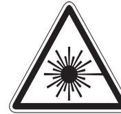
CAUTION - CLASS 3B. INVISIBLE LASER RADIATION WHEN OPEN. AVOID EXPOSURE TO THE BEAM.
