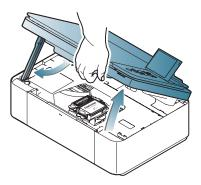
The ink cartridges are located in the printhead.
