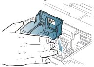
Push firmly against the target label of the printhead until you hear a loud snap.
