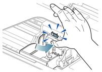
Insert the black ink cartridge into the printhead.
