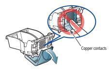
**IMPORTANT**: Be careful not to scratch or touch the copper contacts while inserting the printhead.
