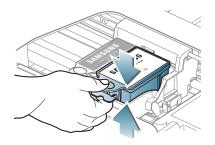
**5** Lift the ink cartridge out of the printhead.
