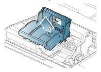
**6** Remove the new printhead from its bag.
