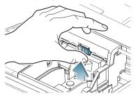
**5** Lift the used printhead out of the carriage.
