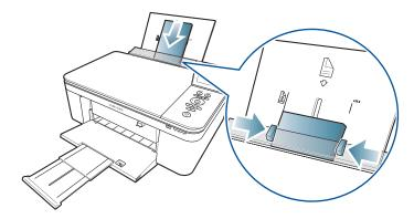
IMPORTANT: Always load the paper **short side first**. The printer automatically detects the orientation of the picture, whether it's portrait or landscape, and prints accordingly. If the photo paper is loaded in the wrong direction, the image will be cut off and the paper may jam. If the paper is loaded with the wrong side up, the image quality will be affected.
