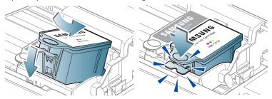
13 Close the printer access door. The printer detects the new printhead. Follow the instructions on the LCD to calibrate your printer.
