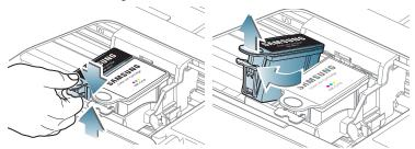
Unlatch the used printhead by lifting the button in the center of the carriage.
