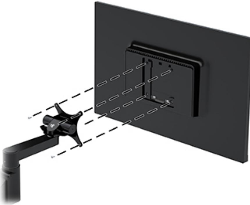
An optional HP Quick Release mounting bracket is available from HP for mounting the monitor. The HP Quick Release connects to the VESA-standard mounting points, allowing you to mount the monitor in a variety of orientations.
