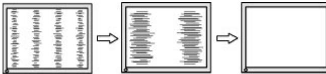
3. After adjusting the Clock, if blurring, flickering, or bars appear on the screen, proceed to adjust the Phase.
