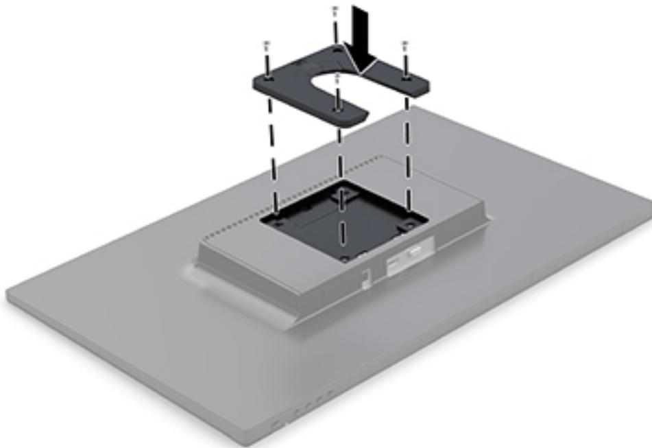
3. Using four screws included in the mounting device kit, attach the other side of the HP Quick Release to the device or surface to which you will mount the monitor. Make sure the release lever points upward.
