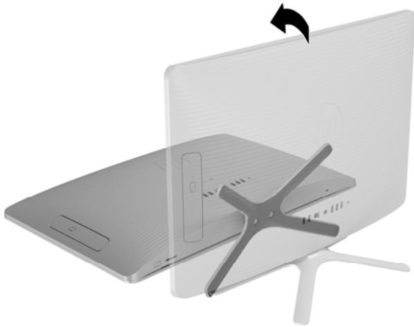
3. To remove the stand, loosen the two captive screws in the bottom of the stand, and then remove the stand from the computer.
