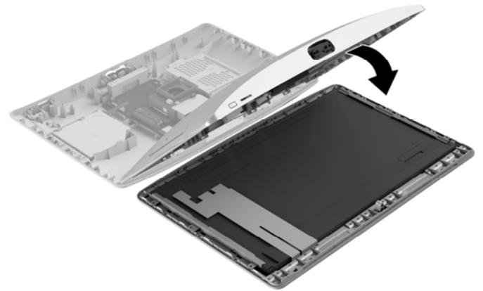
3. Align the cover with the computer and press it down until it snaps into place.
