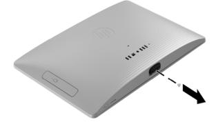
6. To avoid damaging the cable that connects the system board to the rear cover, carefully lift the bottom edge of the cover, and then rotate the cover until it rests upside down next to the display assembly.
