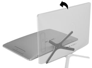
4. To remove the rear cover, remove the Phillips screw located at the bottom of the cover
