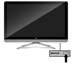
6. Plug the power cord and any additional cables into the back of the computer.
