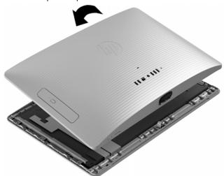
2. Grasp the bottom edge of the cover and carefully rotate the cover toward the display assembly.
