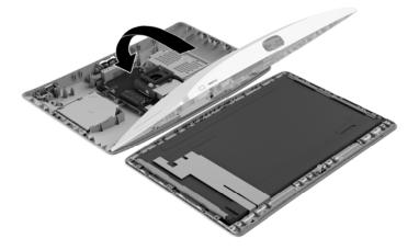
3. To remove the stand, loosen the two captive screws in the bottom of the stand, and then remove the stand from the computer.
