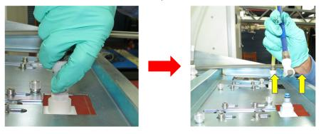
4. Open the two thumbscrews that secure the filter bracket.
