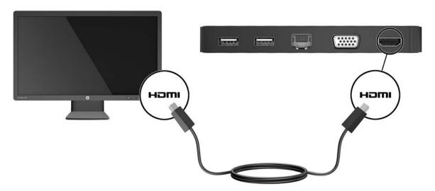
Connect the other end of the cable to the high-definition TV or monitor.
