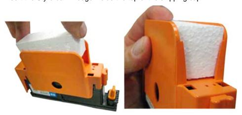
d. Place the printhead inside the bubble-wrap bag.
