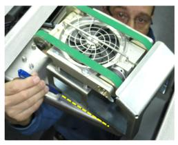
**4.** Using an Allen wrench, remove the 3 screws that secure the Tornado assembly to the OPV interface.
