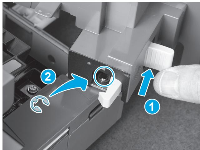
**EN** Keep the latch depressed, and then install the e-ring.
