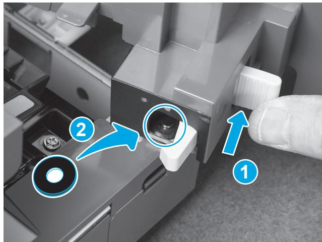
**EN** Keep the latch depressed, and then install the washer.
