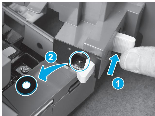
**EN** Keep the latch depressed, and then remove the washer.
