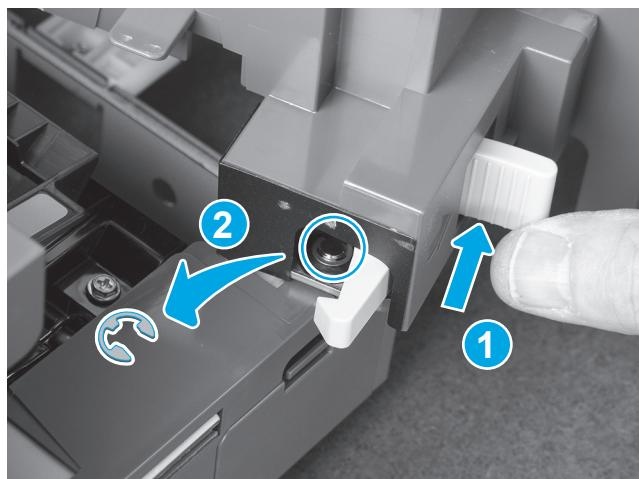
EN Keep the latch depressed, and then remove the e-ring.
