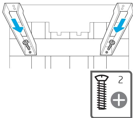
**EN** **8.1** Install the two metal brackets in the slots on the finisher chassis plate, and then install the two smaller screws to fasten the brackets to the finisher.
