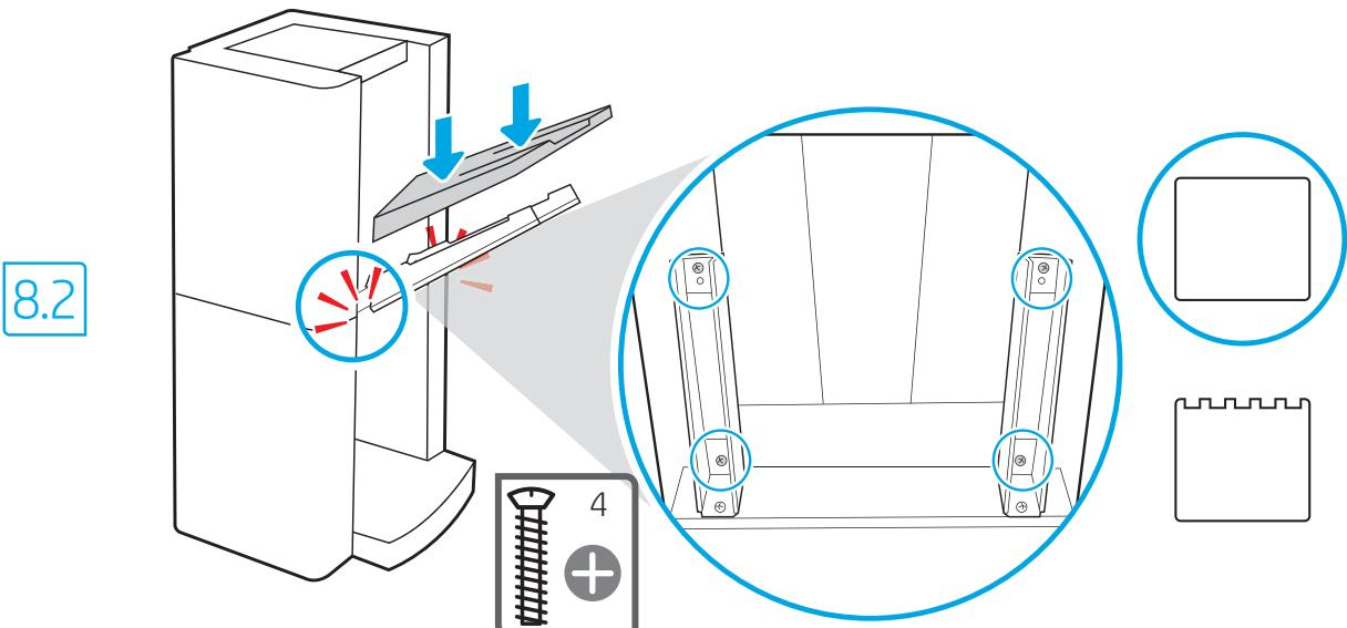
**EN** **8.2** Place the lower output bin on the brackets, press down to align the four screw holes in the bin with the holes in the brackets, and then install the four larger screws.
