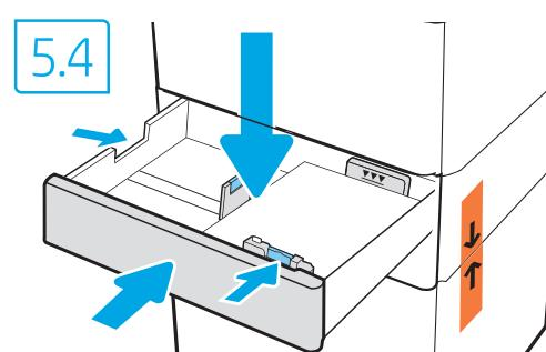
**EN** **CAUTION:** Use Letter/A4 paper in Tray 2 to initialize the printer. The printer will not initialize correctly with Tabloid/A3 paper loaded in Tray 2.
