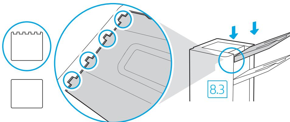
**EN** **8.3** To install the top output bin, align the four tabs on the edge of the bin, with the four slots in the finisher. Insert the tabs with the far end of the bin lifted up, and then once the tabs are inserted, carefully lower the far end of the bin into position.
