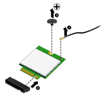
To install the WLAN module, reverse the removal procedures.
