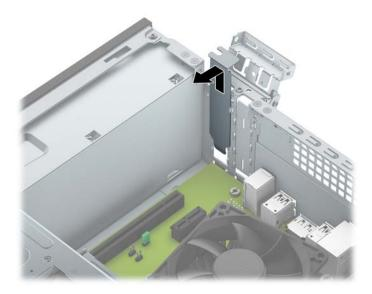
**b.** If you are installing an expansion card in a vacant PCI Express x1 socket, insert a flatblade screwdriver into the slots on the rear of expansion slot cover (1) and rock the slot cover back and forth to break it free from the chassis (2).
