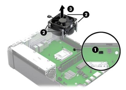
To install the fan sink, reverse the removal procedure.
