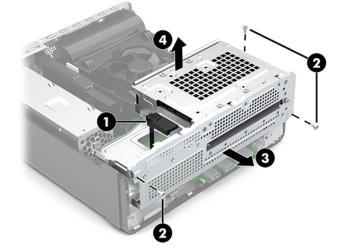
**9.** To remove a hard drive from the drive cage, remove the four screws that secure the drive to the drive cage **(1)**, and then slide the drive out of the cage **(2)**.
