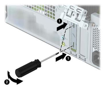
**c.** If you are removing a PCI Express x1 card, hold the card at each end, and carefully rock it back and forth until the connectors pull free from the socket. Pull the expansion card straight up from the socket.
