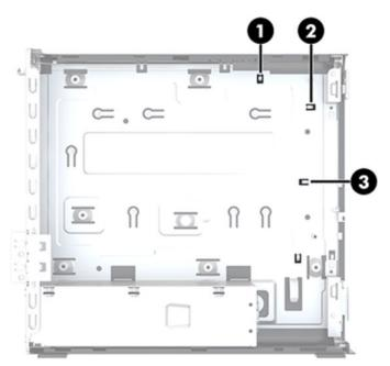
**10.** Peel the antenna off the front of the computer.
