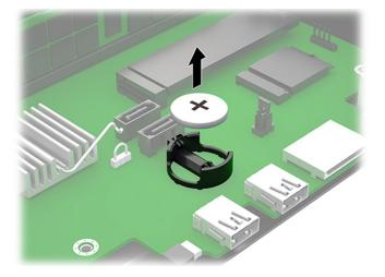
**7.** Slide the replacement battery into position, positive side up. The battery holder automatically secures the battery in the proper position.
