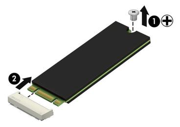
To install the solid-state drive module, reverse the removal procedures.
