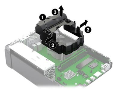
To install the fan duct, reverse the removal procedures.
