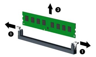
7. To install a memory module, open both latches of the memory module socket (1), and insert the memory module into the socket (2).
