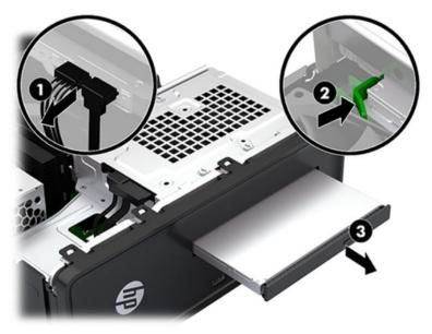
To install the optical drive, reverse the removal procedure.
