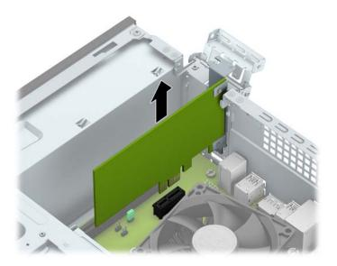
**d.** If you are removing a PCI Express x16 card, pull the retention arm on the back of the expansion socket away from the card (1) and carefully rock the card back and forth until the connectors pull free from the socket. Pull the expansion card straight up from the socket (2).
