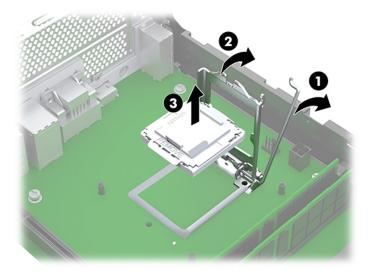
To install a processor, reverse the removal procedure.
