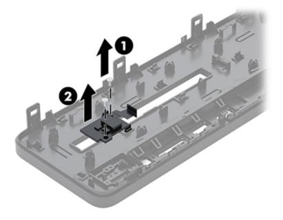
To install the power button board, reverse the removal procedures.
