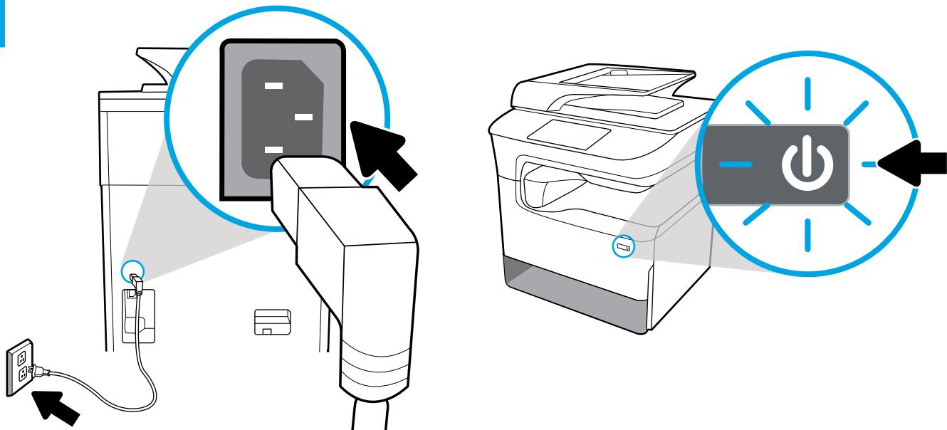
**EN** Connect power cord to AC outlet. Turn on printer.
