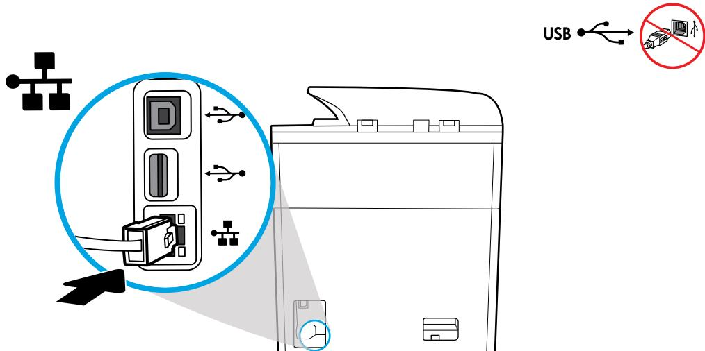
**EN** Connect Ethernet cable, if you want Ethernet connection to network. **Do not connect USB cable at this time.**
