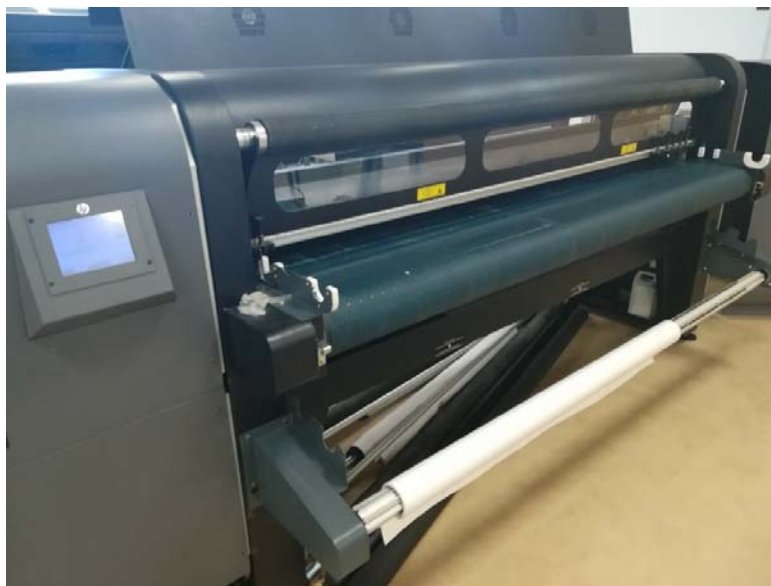
Fig. 3. Manually load the media on the input spindle or use a carriage/forklift to do so.
