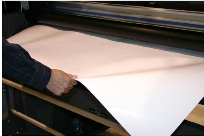
Fig. 6. Pull the media by hand until it reaches the takeup.
