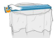
NOTE: The knobs should never be fully unscrewed. This avoids the risk of a loose adjustment plate that could fall and possibly damage your hands.
