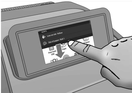
The front panel has a large central area to display dynamic information and icons. On the left side you can see three fixed icons at different times. Normally they are not all displayed at the same time.
