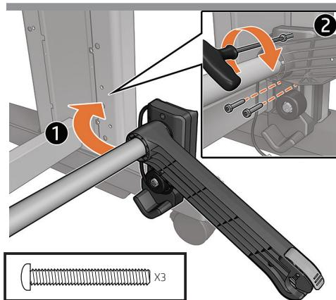
**EN** Slide the pivot block and spacer into the 3 holes of the leg and fix with 3 screws.
