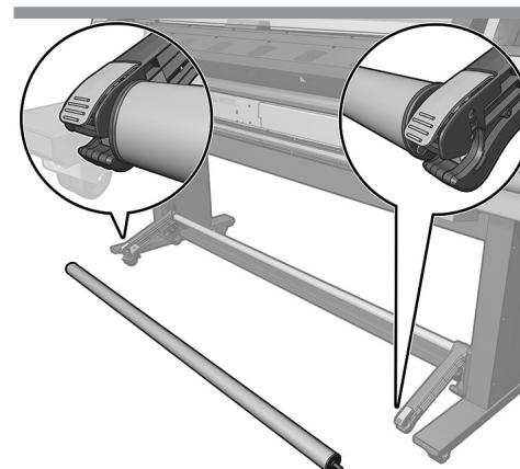
**EN** Slot the loop shaper bar into place.
