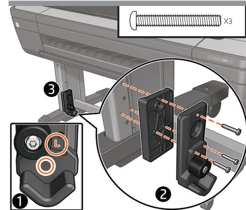
**EN** Attach the left spacer and pivot block (marked with "L") onto the left hand leg and fix with 3 screws.
