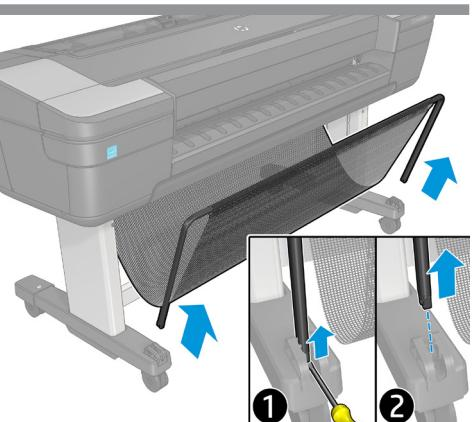
**EN** Unclip the frame from the feet and remove the basket.
