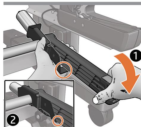
**EN** Pull the tension arm down and make sure it fits inside the arm of the counterweight.
