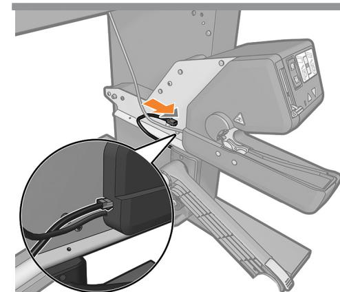
**EN** Connect the cable from the tension bar right support, to the right part of the take up reel.
