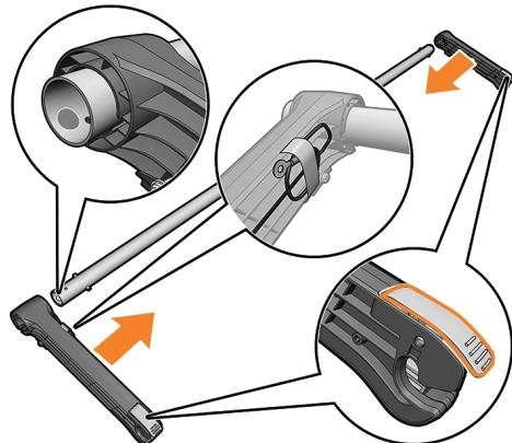
**EN** Slot the two loop shaper arms onto the bar. Make sure the left arm (the one with the cable) is attached to the left side of the bar (green label seen inside the tube) and that the grounding cable is on the inside. Ensure the 2 blue handles are in the up position.
