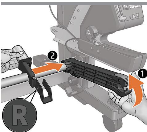
**EN** Install the right counterweight onto the right arm of the tension bar, by moving the arm upwards.
