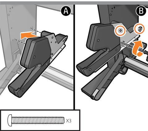
**EN** Identify the 3 holes on the inside left leg and attach the take up reel left hand module into the holes using 3 screws.
