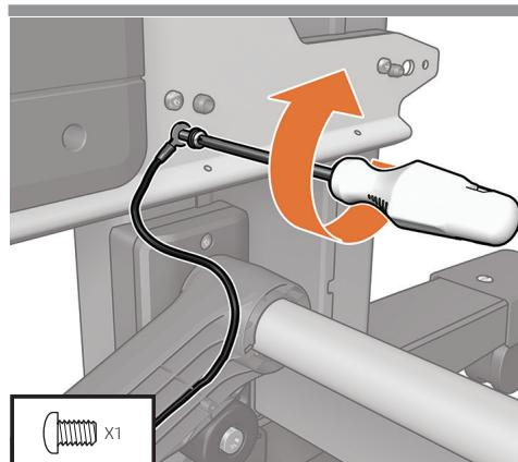
**EN** Use the screw to attach the grounding cable to the leg.
