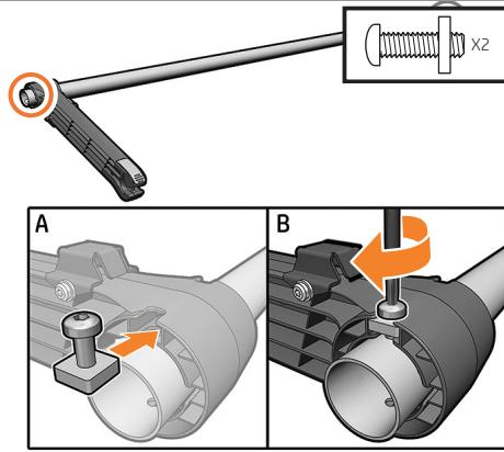
**EN** Slot the 2 square nutted screws into place, and screw in until fully located.
