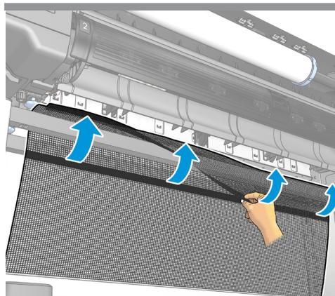
**EN** Before installation, remove the basket from the printer. Pull out the fabric from the bar.
