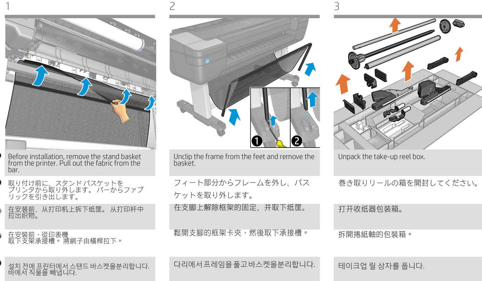
EN Before installation, remove the stand basket from the printer. Pull out the fabric from the bar.
