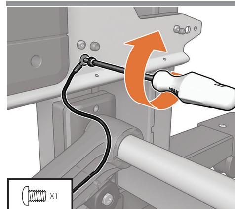
Use the screw to attach the grounding cable to the leg
