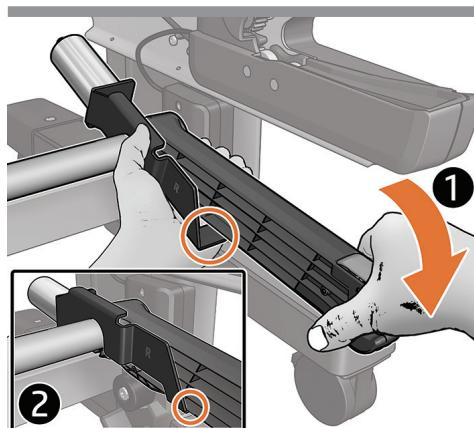
Pull the tension arm down and make sure it fits inside the arm of the counterweight
