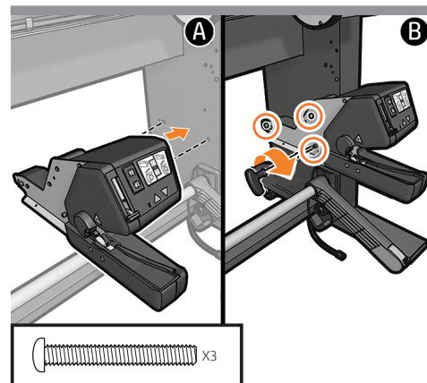
**EN** Attach the right part of the take-up reel module (the one with the cable) to the right leg with 3 screws.
