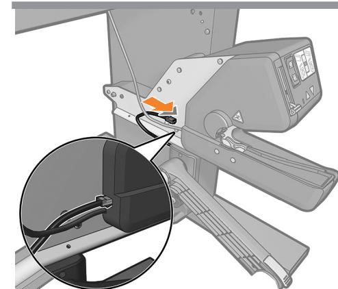
Connect the cable from the tension bar right support, to the right part of the take up reel.
