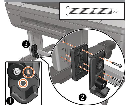
Attach the left spacer and pivot block (marked with "L") onto the left hand leg and fix with 3 screws.
