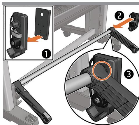
**EN** Attach the right pivot block and spacer onto the other side of the loop shaper.
