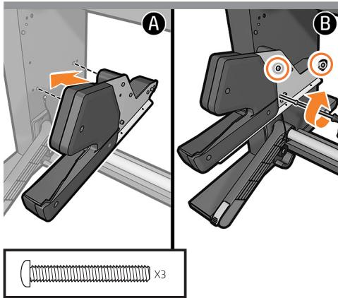
**EN** Identify the 3 holes on the inside left leg and attach the take up reel left hand module into the holes using 3 screws.
