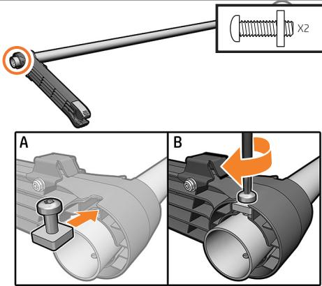
Slot the 2 square nutted screws into place, and screw in until fully located.
