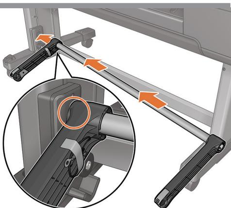
**EN** Insert the loop shaper into the left hand side pivot block.
