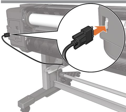
**EN** Connect the cable to the port at the rear of the printer.
