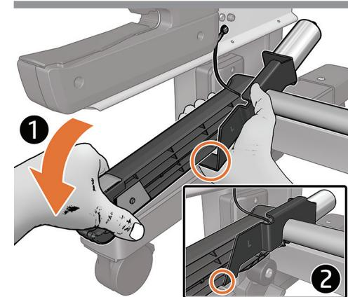
**EN** Pull the tension arm down and make sure it fits inside the arm of the counterweight.
