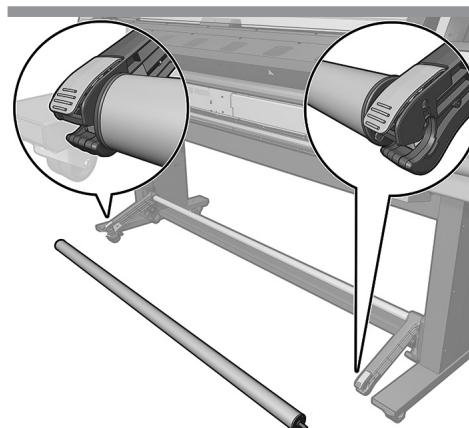
Slot the loop shaper bar into place.
