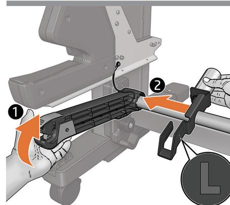
**EN** Install the left counterweight onto the left arm of the tension bar by moving the arm upwards.
