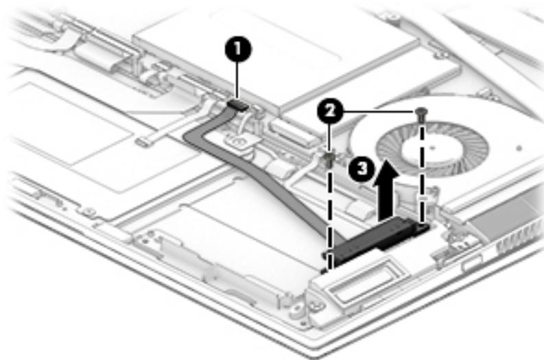
Reverse this procedure to install the drive connector.
