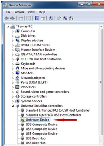
7. Test USB device on a verified working computer to make sure USB device is not malfunctioning.
