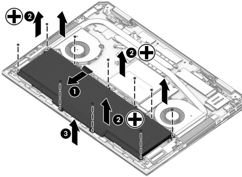
Reverse this procedure to install the battery.
