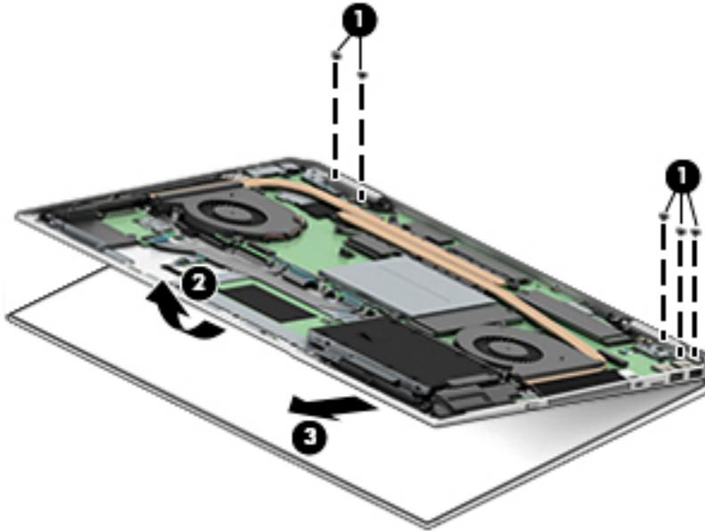
8. If it is necessary to replace any of the display assembly subcomponents:
