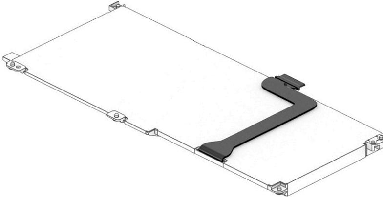
**6-cell battery cable routing**
