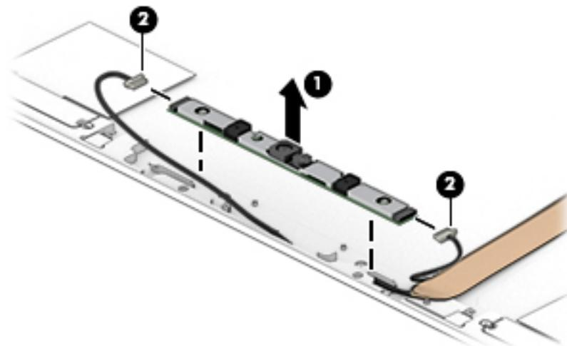
The camera module is available using spare part number L30660-001 for IR cameras.
