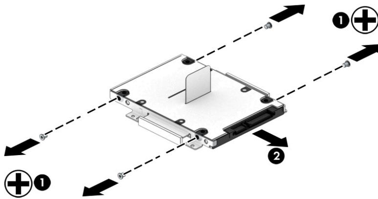
Reverse this procedure to reassemble and install the solid-state drive.
