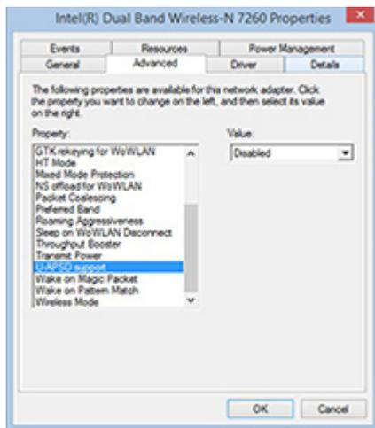
In the example to the left, **U-APSD support** (Unscheduled Automatic Power Save Delivery) is changed to **Disabled** to resolve an incompatible access point. If disabling U-APSD improves the throughput issue, check with the access point provider for updated firmware that resolves the issue.
