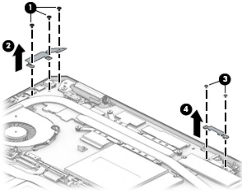
Brackets are available in the Bracket Kit using spare part number L28674-001.
