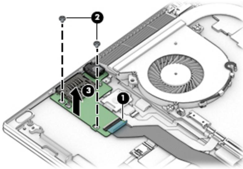
Reverse this procedure to install the card reader/audio board.
