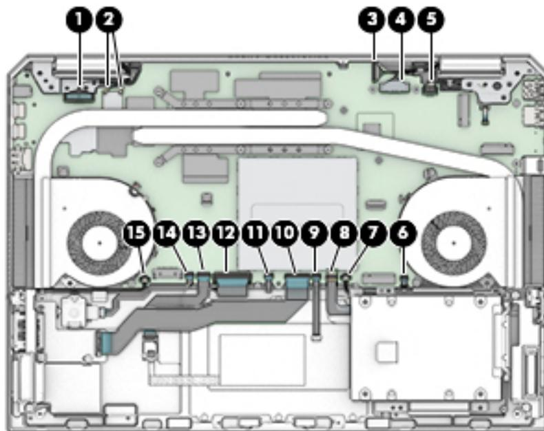
4. Remove the two Phillips M2.0×4.0 screws (2) from each fan.
