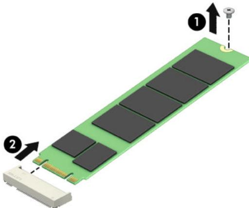
Reverse this procedure to install the Optane memory module.
