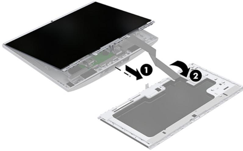
Reverse this procedure to install the display.
