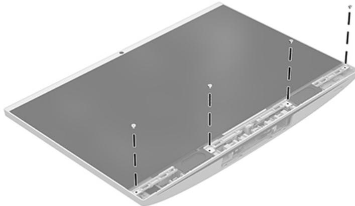
7. Remove the Phillips screw under the stand that secures the display to the computer **(1)**.
