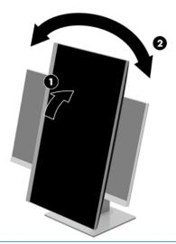
NOTE: To view information on the screen in portrait mode, you can install the HP Display Assistant software included on the software and documentation optical disc or download from <a href="https://www.hp.com/support">www.hp.com/support</a>. The position of the OSD menu can also be rotated to portrait mode. To rotate the OSD menu, access the OSD menu by pressing the Menu button on the front bezel, select OSD Control from the menu, and then select OSD Rotation.
