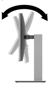
2. Swivel the monitor panel to the left or right for the best viewing angle.
