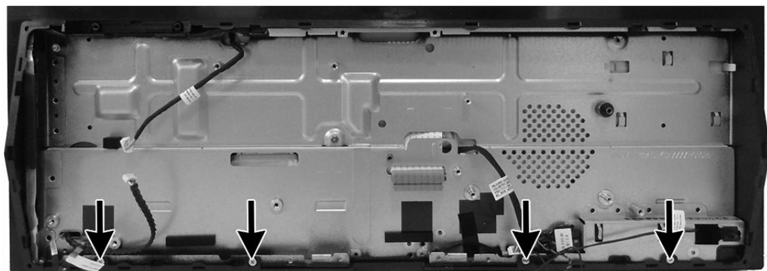
11. Starting near the bottom right (as viewed from the rear), pull the rear closure up to disengage it from the computer. Work upward, and then toward the left, lifting the enclosure up to disengage, and then lift the rear enclosure off the computer.
