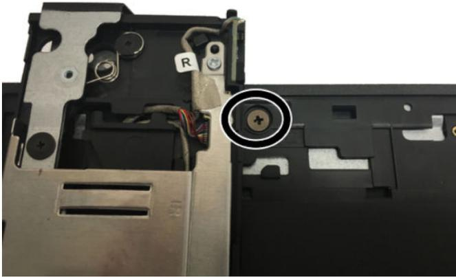
9. From the front of the computer, remove the three Phillips screw located under the speaker cover that secure the rear enclosure to the computer.
