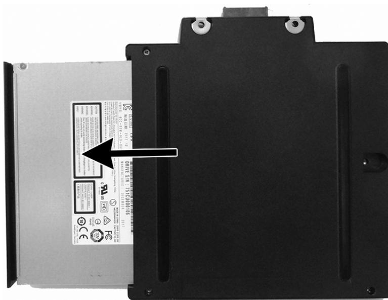
Reverse the removal procedures to install an optical drive.
