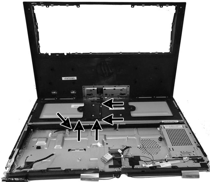
13. To remove the main chassis, remove the four Phillips screws around the sides (1) and the Phillips screw in the middle (2) of the chassis.
