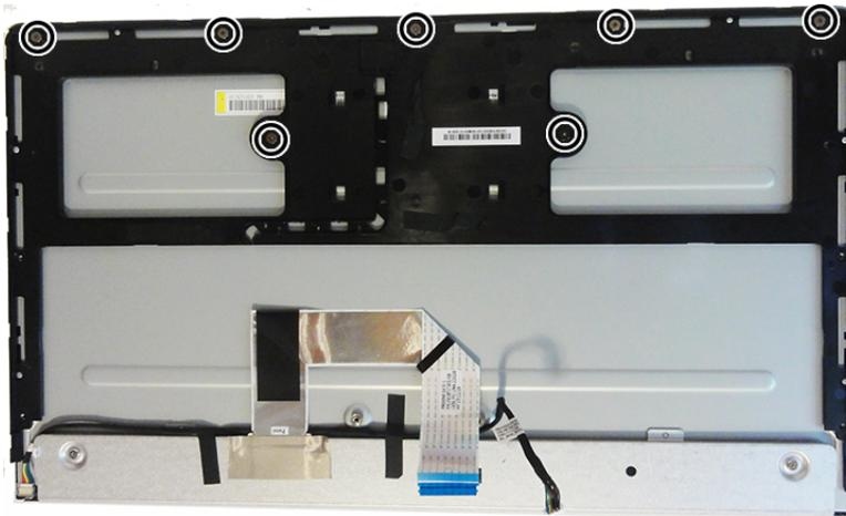
**IMPORTANT:** Install the new display panel together with all other parts in the replacement kit. Do not reuse any old parts. Return all old parts to HP for warranty processing.
