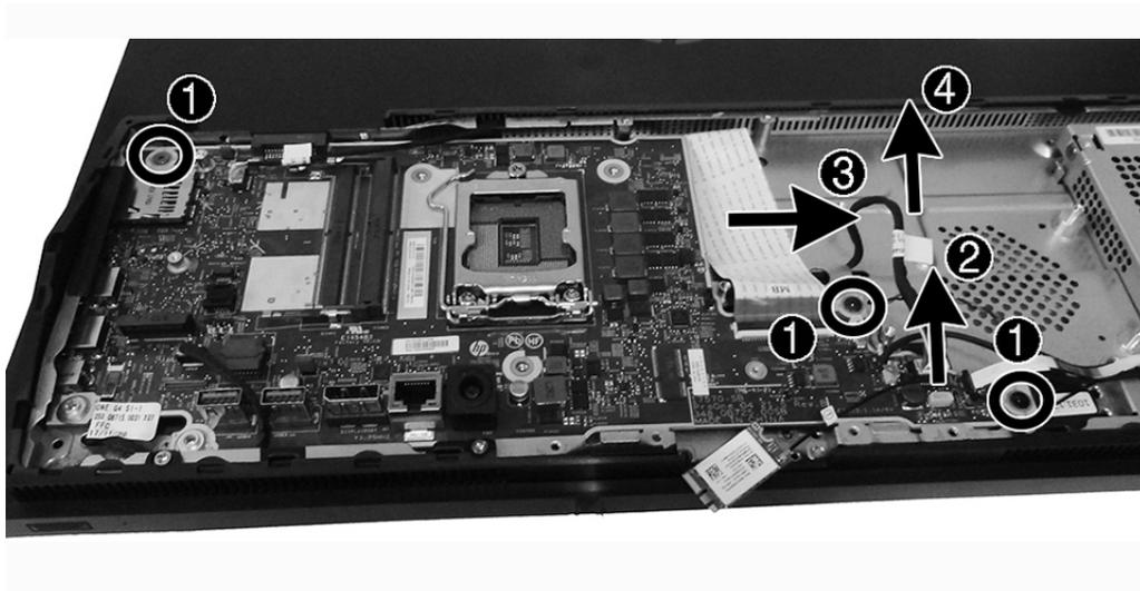
To install the system board, reverse the removal procedures.
