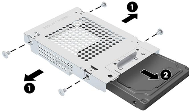
Reverse the removal procedures to install a hard drive.
