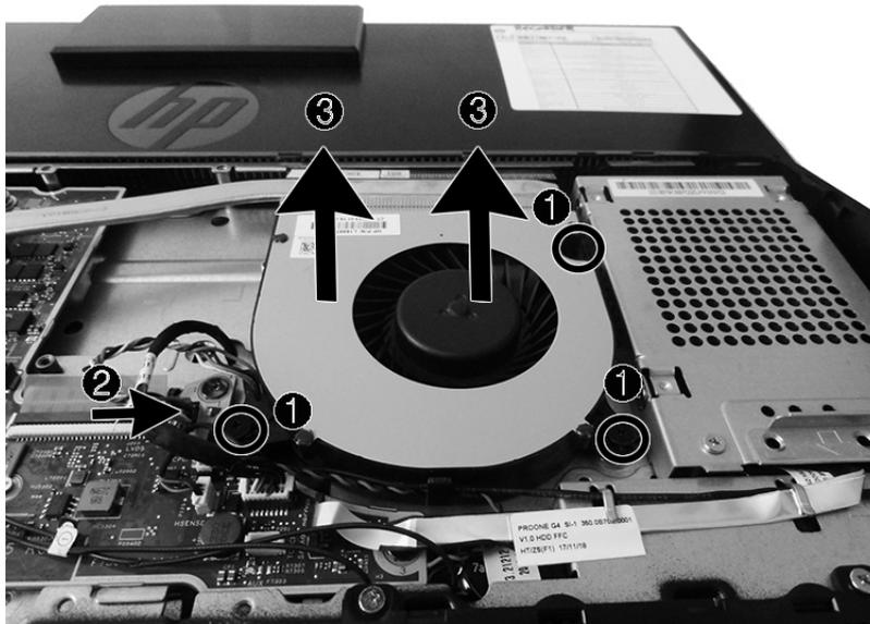
To install the fan assembly, reverse the removal procedures.
