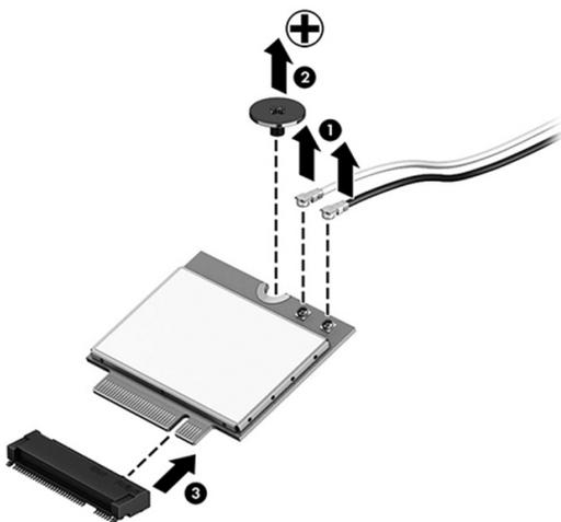
To install the WLAN module, reverse the removal procedures.
