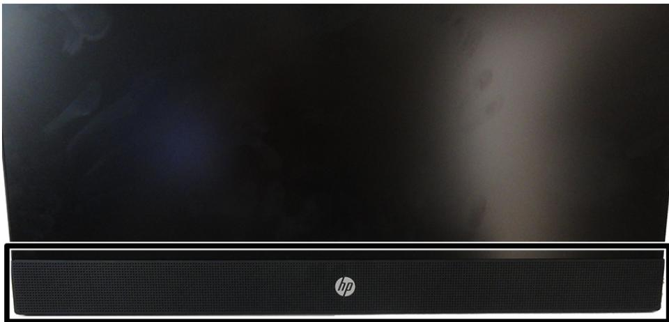
5. Rotate the top of the cover downward to disengage the snaps from the chassis, and then remove the cover.
