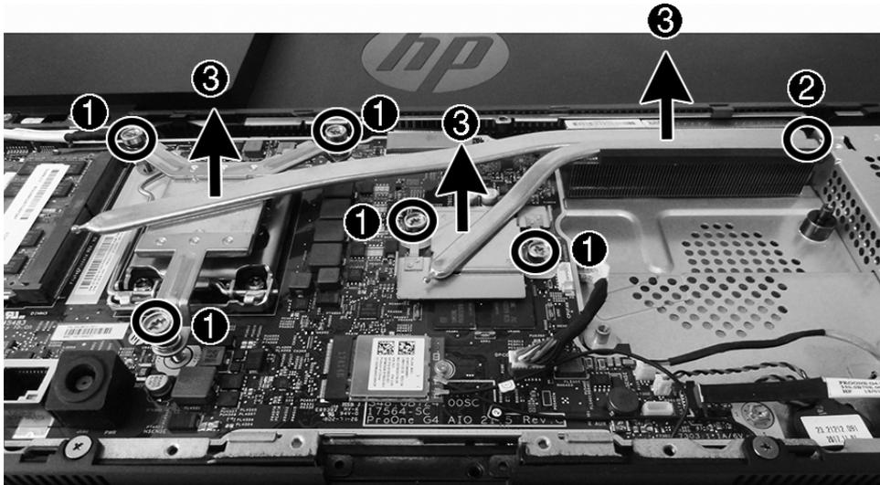
To replace the heat sink, reverse the removal procedures.
