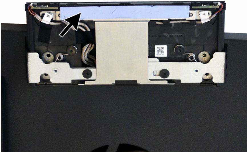
5. Remove the two Phillips screws **(1)** that secure the webcam, and then disconnect the cable from the webcam **(2)**.
