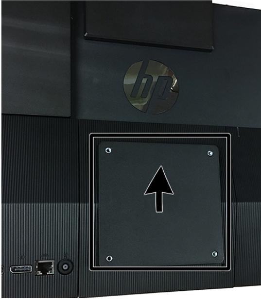
3. Remove the two screws (1) that secure the VESA bracket to the computer.
