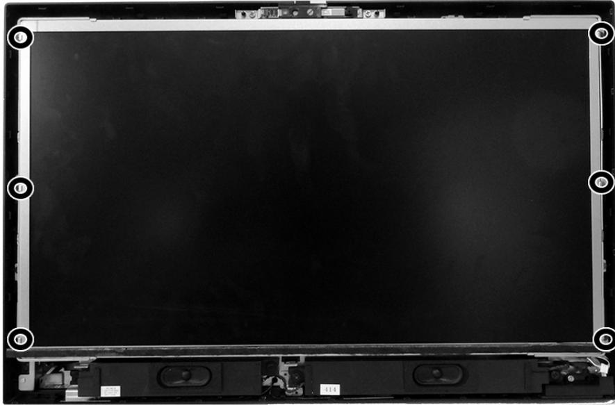
9. Disconnect the main display cable from the rear of the display panel (1), and disconnect the backlight cable from the display panel (2).
