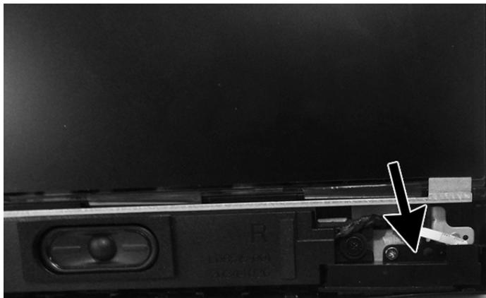
7. Remove Phillips screw **(1)** that secures the power button board to the computer.
