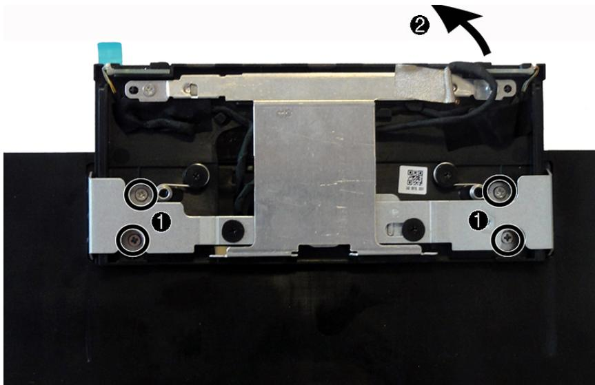
8. Remove the screw from under the webcam.
