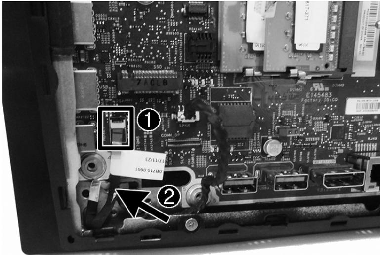
6. Locate the power button board under the speaker cover.
