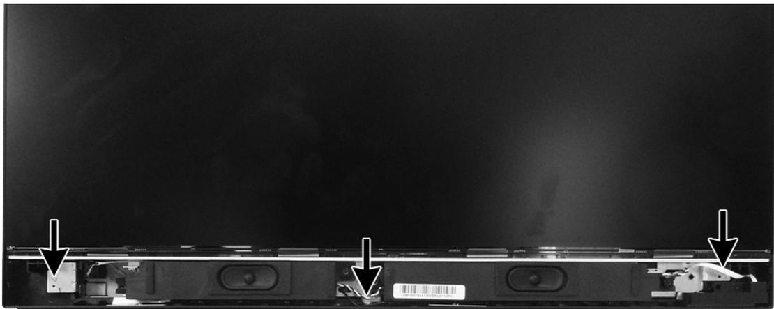
10. From the rear of the computer, remove the four Phillips screw located along the bottom edge of the computer.
