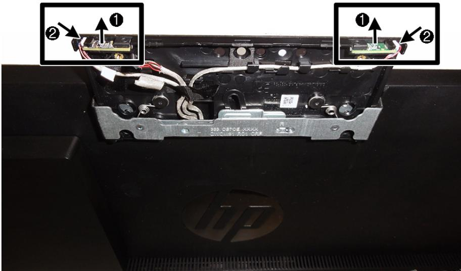
To install webcam and microphone modules reverse the removal procedures.
