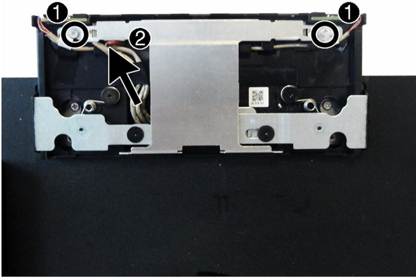
6. Remove the webcam and bracket from the computer.
