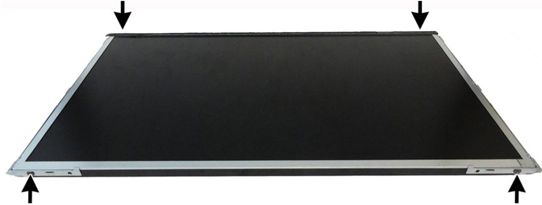
12. Pull the brackets off the sides of the display panel.
