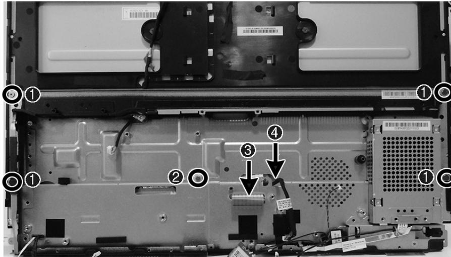
15. Remove the chassis from the display panel.
