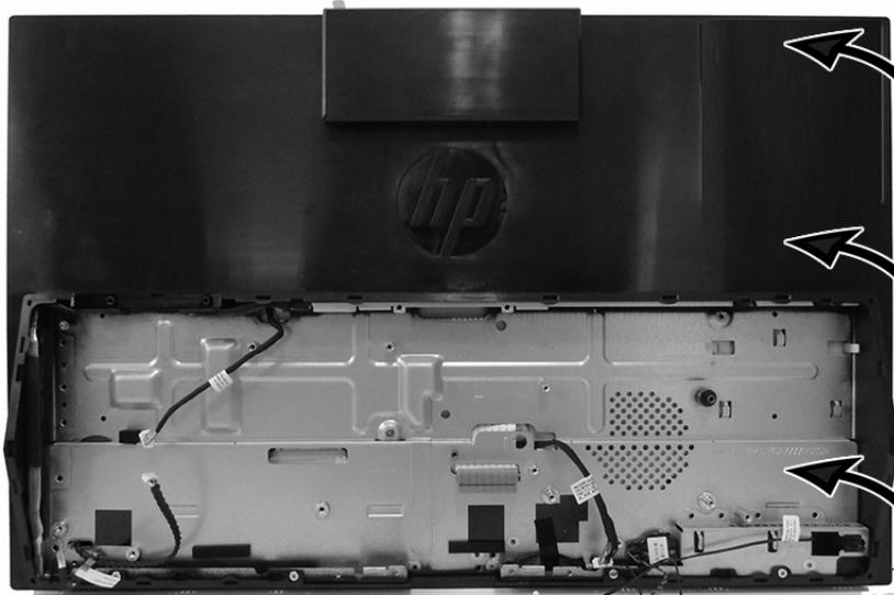
12. Position the rear enclosure next to the computer. Note proper webcam cable routing, as pointing out in the following image. The webcam cable routes across the display panel and then under the chassis. You must remove the chassis from the panel to remove the webcam cable.
