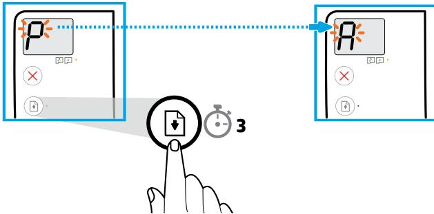
Press (Resume) for 3 seconds. Wait for alignment page to print when blinking “P” becomes “A”.
