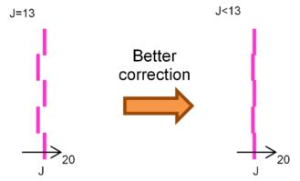
In this case, the diagram shows that we need to change the value corresponding to the J pattern. Also it indicates that the correction needs to be moved towards lower values, because the '20' value would move it in the wrong direction.
