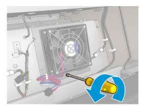
**6.** Remove the fan-resistor module.
