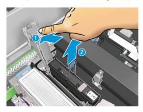
If the printhead is to be reused, protect it using its orange sealing cap.
