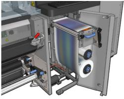
Pull the black knob on the upper left and move the pinch system aside.
