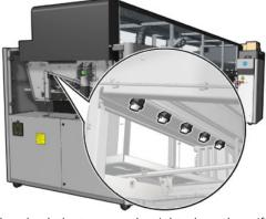
Also check the trays on the right; clean them if necessary by absorbing the oil with a cloth or other absorbent material.
