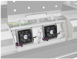
Disconnect the two cables shown in the picture. You have to press the retention clip on each of the two connectors, and gently pull the cable. The black one is for the DC fans supply and the white one is for AC power to the curing heaters.
