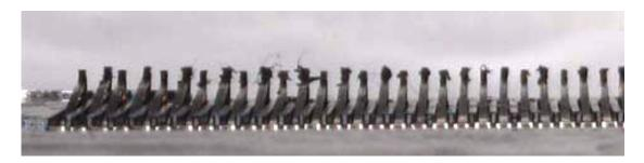
3. Clean the dirty connections gently but thoroughly using the brush provided in the HP Latex 3x00 Printer Cleaning Kit. A piece of paper or cloth can be used to collect the dirt.
