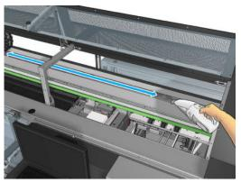
Alternatively, use an absorbent cloth, moistened with deionized water, to wipe off the dust. Ensure that the dust adheres to the cloth and does not fall into the printer.
