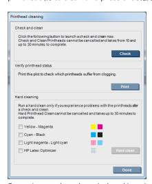
Sometimes, when the printhead is quite damaged, running the hard-clean routine twice helps to recover its performance.
