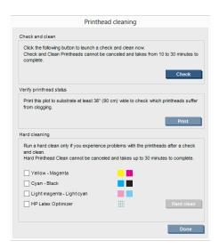
Press the **Check** button to perform routine cleaning automatically.
