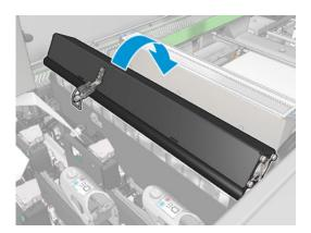
Remove both aerosol filters, using their handles.
