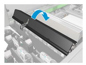
Remove both aerosol filters, using their handles.
