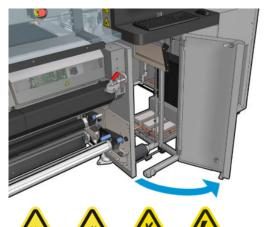
7. Check the front and back collectors visible from the door.
