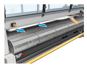
9. Keep the substrate evenly tensioned and push the output rubber spindle backwards. Take care not to trap your fingers between the roller and the black substrate guide lying underneath and behind. Close both latches and the lever.
