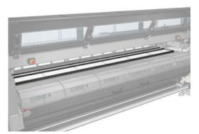
13. Go to the rear of the printer, lower the pinchwheel latches (1), and pull down the pinchwheel module to its lowest position.
