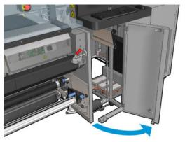
4. Pull out the printhead cleaning roll carriage.
