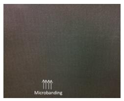
Microbanding is probably caused by a faulty printhead. Print the printhead alignment diagnostics plot (see Printhead alignment diagnostics plot on page 163) to find which printhead is responsible, and replace the printhead.
