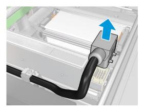
Unscrew the three screws shown below in order to remove the drying module (the left module is shown).
