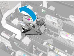
Lift the handle provided with the printhead, and pull the handle gently upwards to disconnect the printhead from the carriage.
