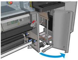
Grip the handle and pull the whole printhead cleaning roll assembly out through the door. 3.
