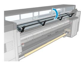
2. Check all of the front collectors at the center of the printer.
