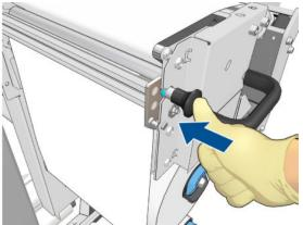
13. Grip the handle and push the whole printhead cleaning roll assembly back into the printer. Ensure that you push it as far as it will go.
