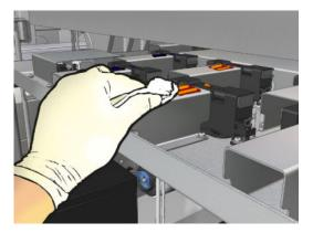
4. Scrub the surface of each ink deposit with the steel scourer, taking care to move it from the inside of the printer towards the outside, to avoid pushing dirt into the drop detector.
