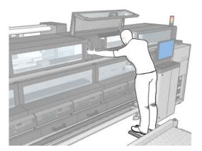
4. Open one latch on the left side of each aerosol filter module.
