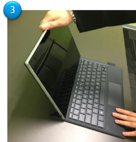
Dock Slate to pogo pin bar on the keyboard rear side
