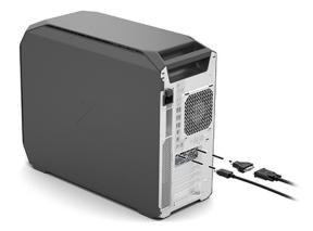
Connect the other ends of the monitor cables to the monitors.
