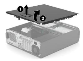
Reverse this procedure to install the access panel.
