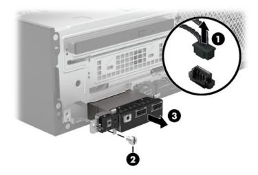
Reverse this procedure to install the FIOUI module.
