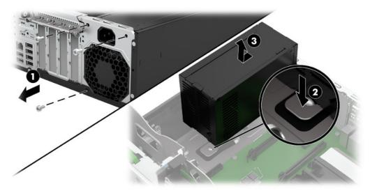
Reverse this procedure to install the power supply.
