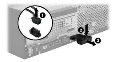
Reverse this procedure to install the SD card reader module.
