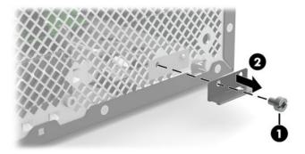
Reverse this procedure to install the front antenna.
