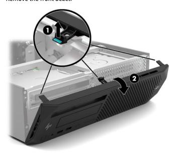
Reverse this procedure to install the front bezel.
