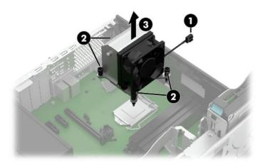
Reverse this procedure to install the CPU cooler.
