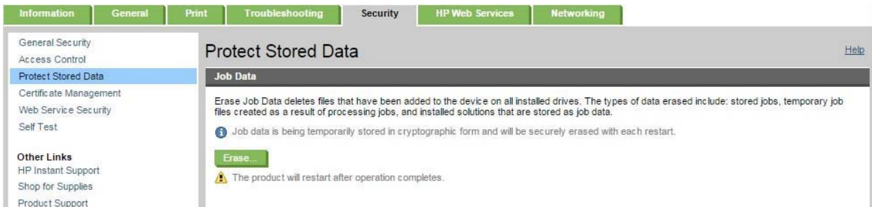
Figure 13: Erase Job Date option using an eMMC system disk in the Embedded Web Server (EWS)
