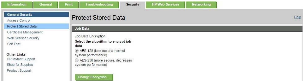
Figure 14: Job Data Encryption using an eMMC system disk in the Embedded Web Server (EWS)
