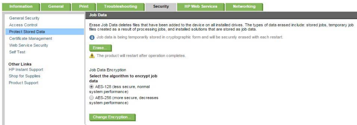
Figure 9: Managing Job Data Encryption on an SSD or eMMC system disk in the Embedded Web Server (EWS)
