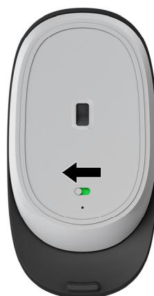
2. Lift the cover off the top of the mouse (1), and then install the batteries (2). Replace the cover.
