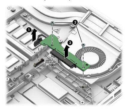
If it is necessary to replace the hard drive connector board cable, after removing the board, disconnect the cable from the board.
