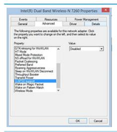
In the example to the left, U-APSD support (Unscheduled Automatic Power Save Delivery) is changed to **Disabled** to resolve an incompatible access point. If disabling U-APSD improves the throughput issue, check with the access point provider for updated firmware that resolves the issue.
