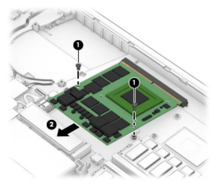
Reverse this procedure to install the discrete graphics board.
