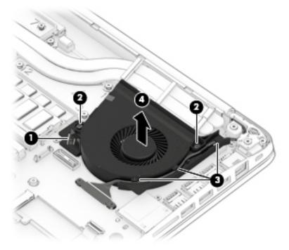
3. Release the fan connection (1) on the GPU fan, and then release the two captive screws (2) securing the GPU fan to the computer.
