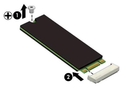
Reverse this procedure to install the solid-state drive.
