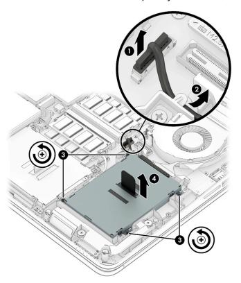
Repeat steps 1 through 4 to remove the secondary hard drive.
