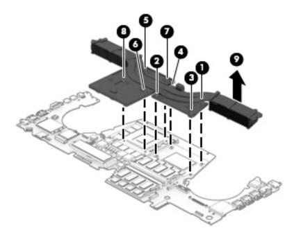
The following illustration shows the replacement thermal material locations. The thermal material must be thoroughly cleaned from the surfaces of the heat sink and the system board components each time the heat sink is removed. Replacement thermal material is included with the heat sink and system board spare part kits.
