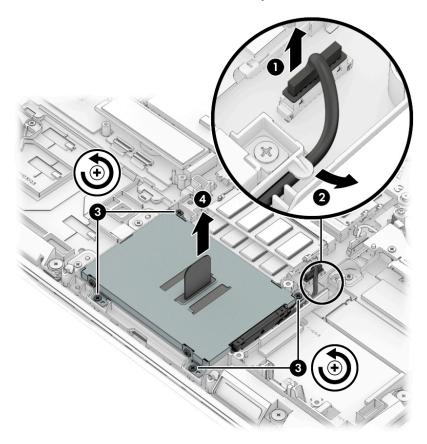
8. If it is necessary to replace the hard drive connector adapter on a hard drive, slide the adapter (1) off of the front end of the hard drive.
