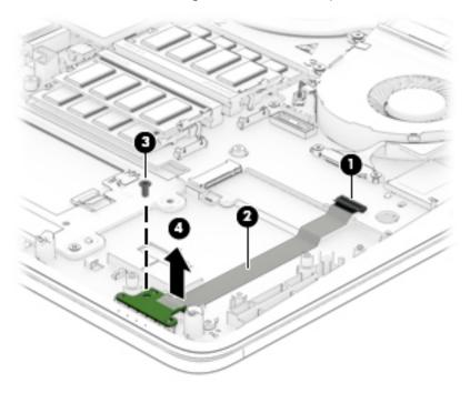
Reverse this procedure to install the display LED board.
