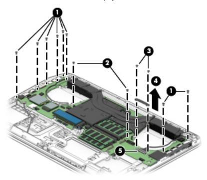
**6.** Lift the side of the system board **(1)** and slide system board **(2)** at angle away from the computer to remove it.
