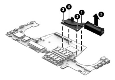
The following illustration shows the replacement thermal material locations. The thermal material must be thoroughly cleaned from the surfaces of the heat sink and the system board components each time the heat sink is removed. Replacement thermal material is included with the heat sink and system board spare part kits.
