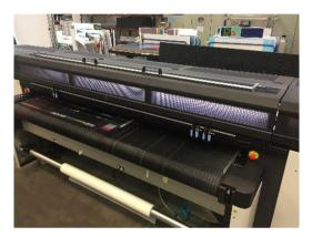
2. Lift up the side alignment bars on both sides.
