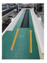
7. Place the new velvet with the rods inside the beam slots.
