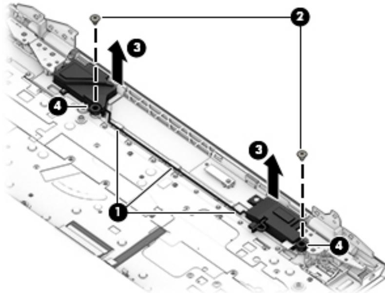
Reverse this procedure to install the rear speakers.
