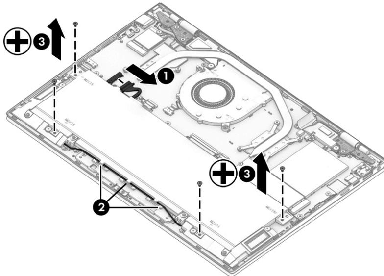
4. Release the battery **(1)** by sliding it toward the back of the computer.
