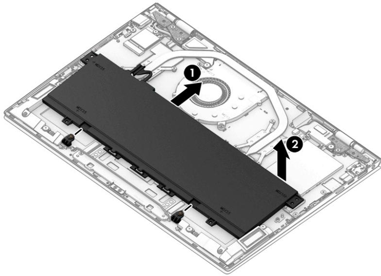
Reverse this procedure to install the battery.
