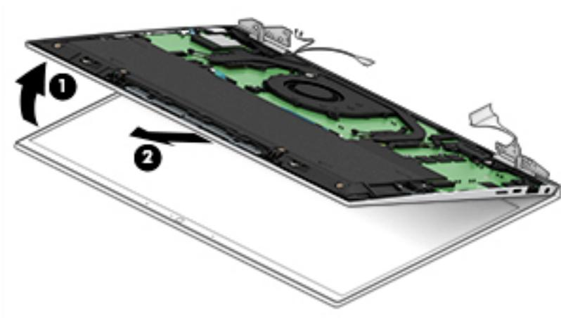
Reverse this procedure to install the display assembly.
