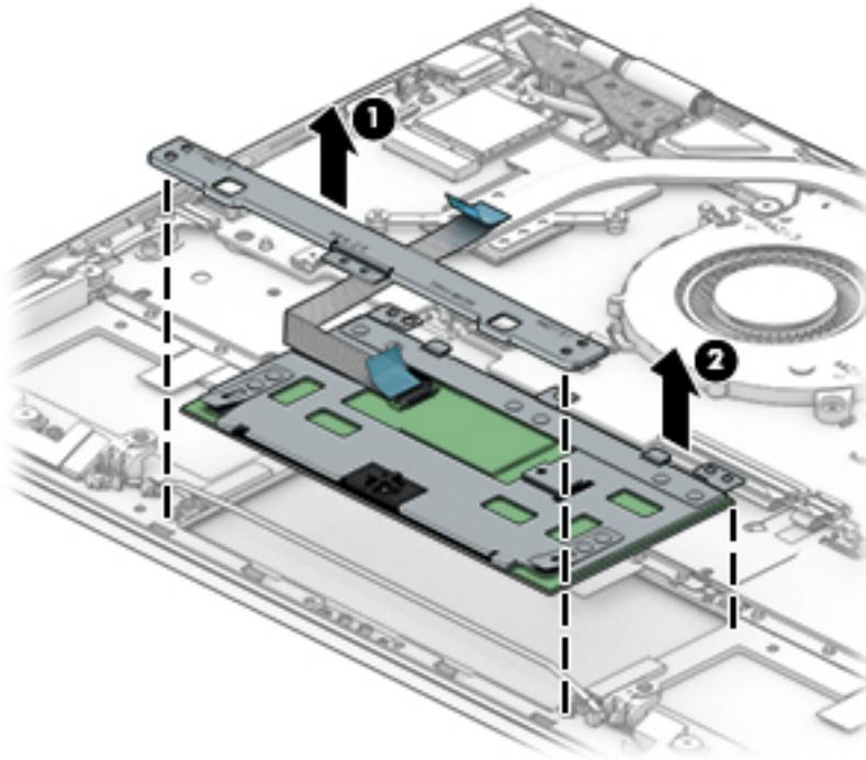
Reverse this procedure to install the TouchPad and bracket.
