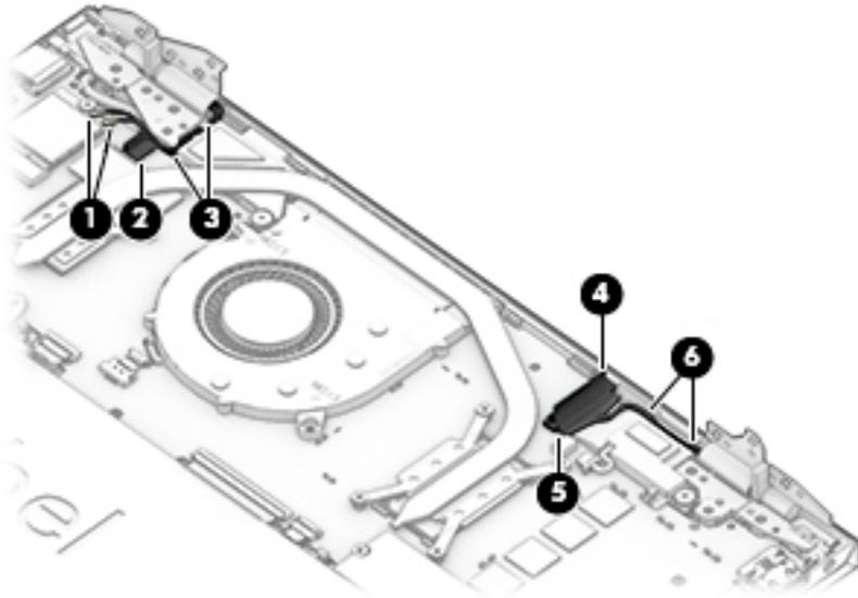
7. Remove the three Phillips M2.5×6.7 screws **(1)** that secure the display hinges to the keyboard/top cover.
