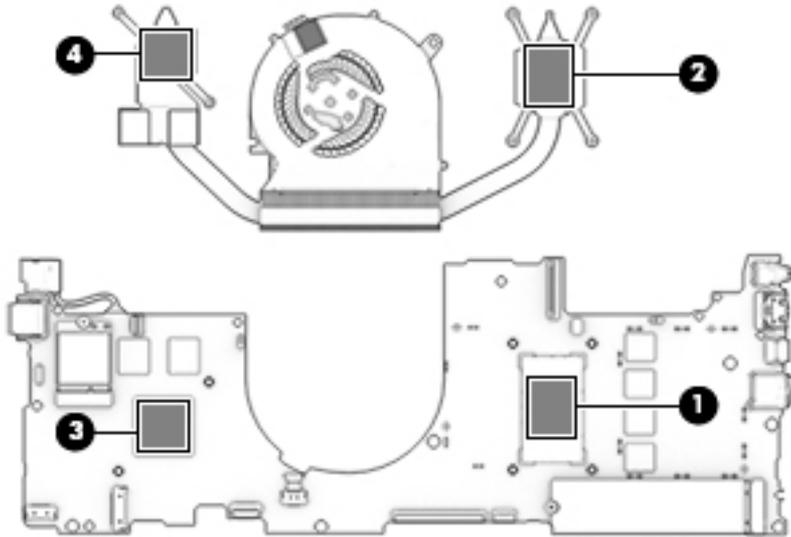
**Computer model equipped with a graphics subsystem with UMA memory:** Thermal paste is used on the processor (1) and the fan/heat sink assembly section (2) that services it.
