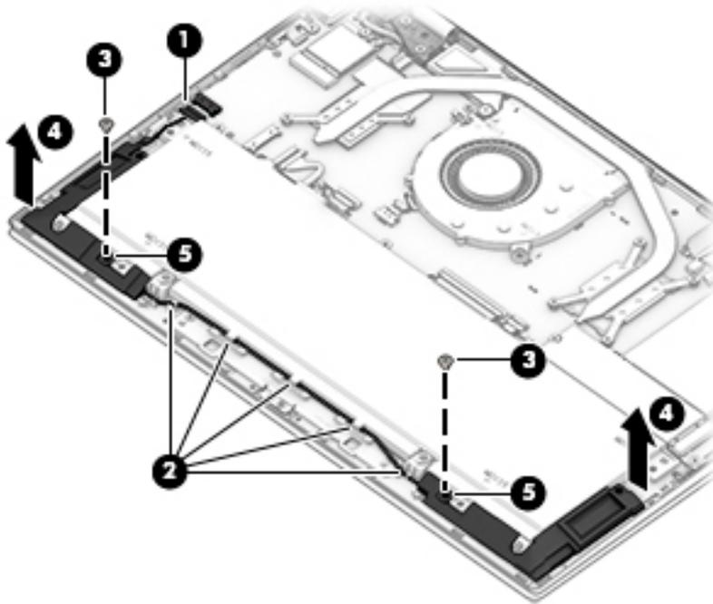
Reverse this procedure to install the front speakers.
