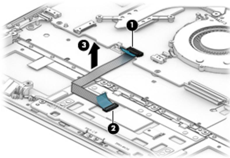
Reverse this procedure to install the TouchPad cable.
