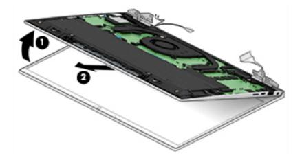
Reverse this procedure to install the display assembly.
