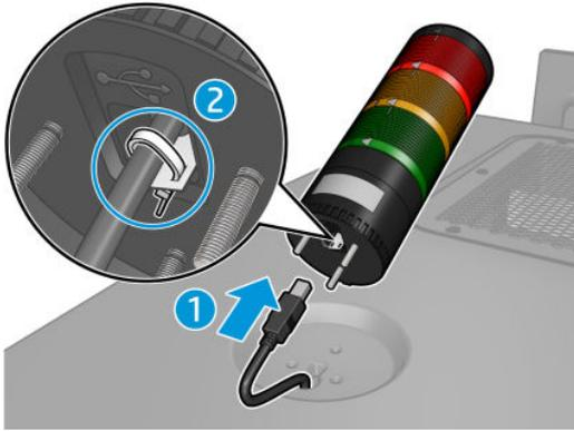
4. Assemble the status beacon, and attach it to the printer using the three provided M4 wing nuts.
