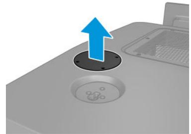
2. Use a Torx-20 screwdriver to unscrew and disassemble the upper and lower back covers.
