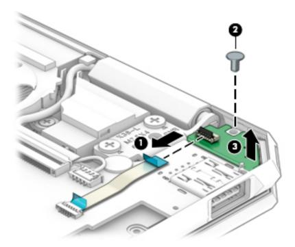
4. Rotate the power button (1), and then remove the power button (2).
