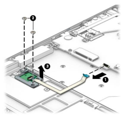
Reverse this procedure to install the fingerprint reader.
