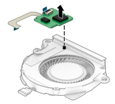
Reverse this procedure to install the IR sensor.
