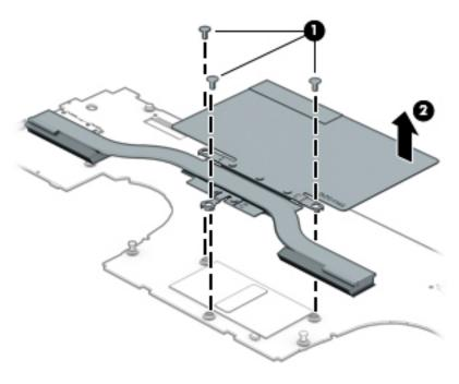
Reverse this procedure to install the heat sink on the system board.
