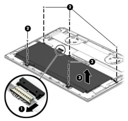
Reverse this procedure to install the battery.
