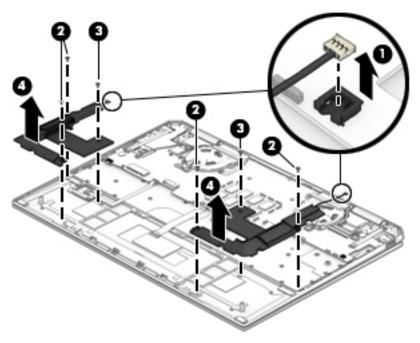
Reverse this procedure to install the front speakers.
