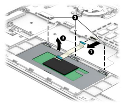
To insert the TouchPad, reverse the removal procedures.
