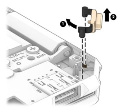
Reverse this procedure to install the power button and the power button board.
