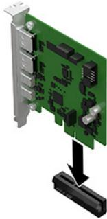
4. Connect the GPIO cable to the connector on the upper-right corner of the card, and then connect the other end of the cable to the system board connector labeled PD129.
