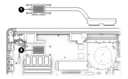
To remove the heat sink assembly from products with discrete graphics:
