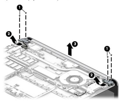
Remove the display assembly subcomponents:
