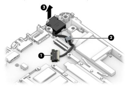
Reverse this procedure to install the power connector cable.
