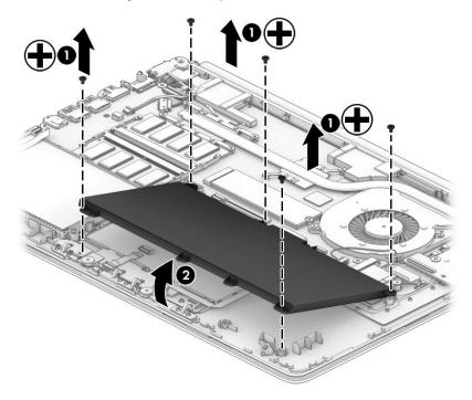
Reverse this procedure to install the battery.
