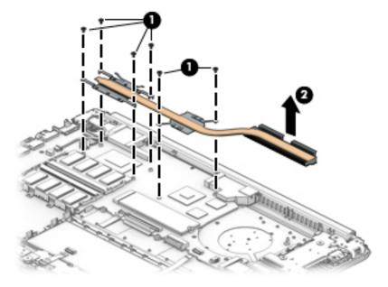
3. Thoroughly clean the thermal material from the surfaces of the heat sink (1)(3) and associated system board components (2)(4) each time the heat sink is removed. Replacement thermal material is included with the heat sink and system board spare part kits.
