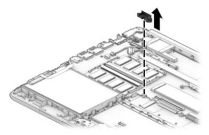
Reverse this procedure to install the system board hook.
