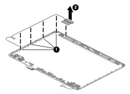
Use the following image to determine proper cable routing in the display of the antenna cable (1) and display cable (2).
