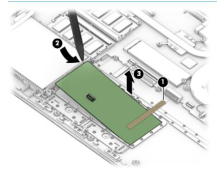
Reverse this procedure to install the TouchPad module.
