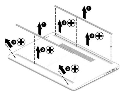
3. Starting near the power connector, use a plastic tool (1) to pry the bottom cover up to remove it (2).
