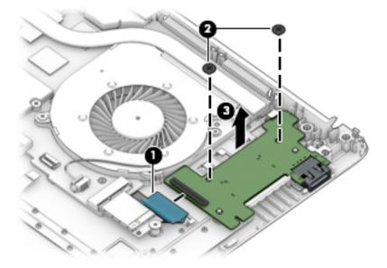
Reverse this procedure to replace the USB/card reader/power button board.
