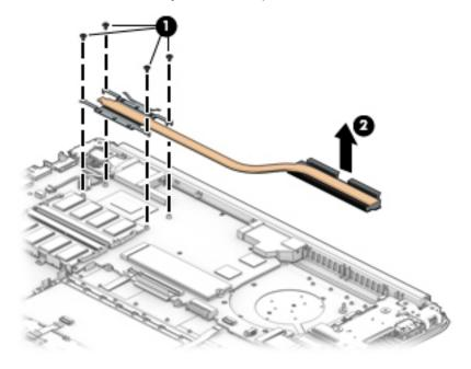
3. Thoroughly clean the thermal material from the surface of the heat sink (1) and associated system board component (2) each time the heat sink is removed. Replacement thermal material is included with the heat sink and system board spare part kits.
