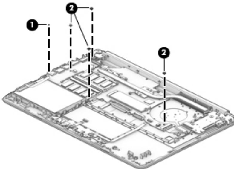
3. Lift the left side of the system board (1), and then remove it from the computer (2).
