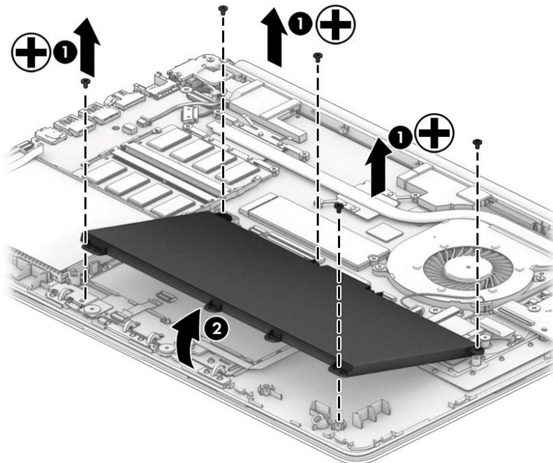
Reverse this procedure to install the battery.
