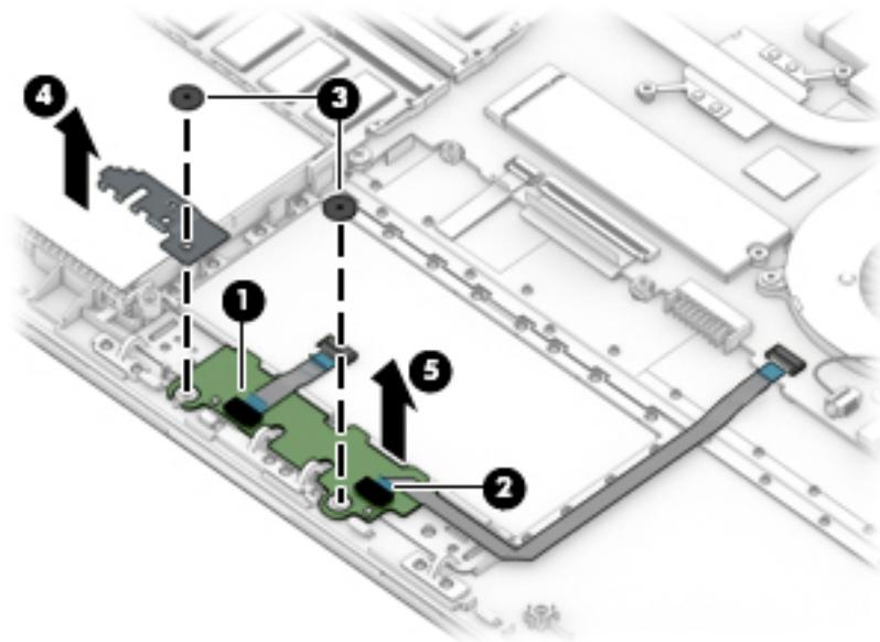
Reverse this procedure to install the TouchPad button board.
