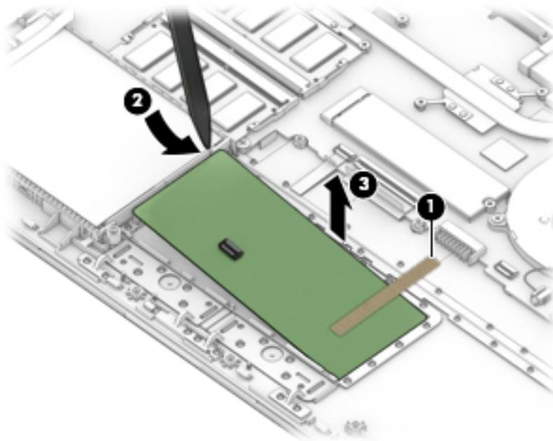
Reverse this procedure to install the TouchPad module.
