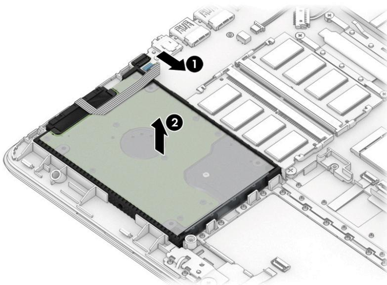
3. If it is necessary to disassemble the hard drive, pull the connector off the rear of the drive **(1)**, and then lift the cover off the drive **(2)**.
