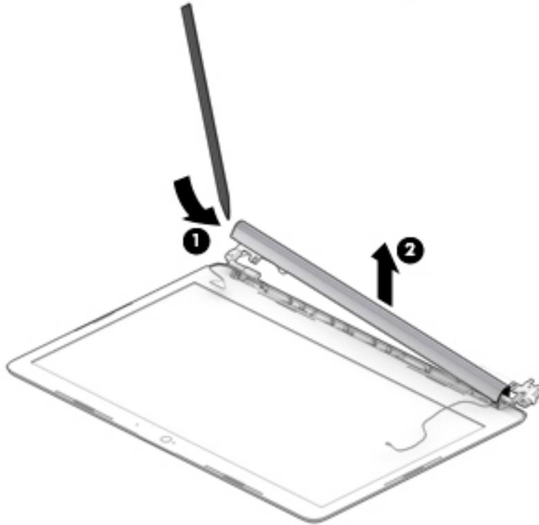
When replacing the hinge cover, make sure the hinges rotate downward as far as they can go. Align the cover **(1)**, and then start from above and rotate the cover downward onto the hinges **(2)**. Make sure the clips snap into place along the bottom of the display cover.
