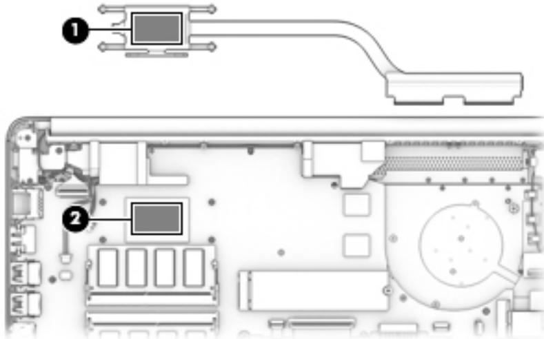
To remove the heat sink assembly from products with discrete graphics:
