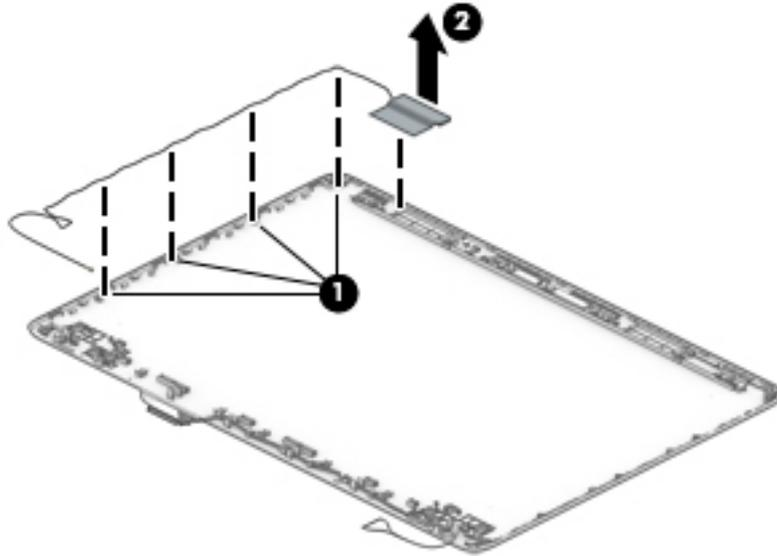
Use the following image to determine proper cable routing in the display of the antenna cable (1) and display cable (2).
