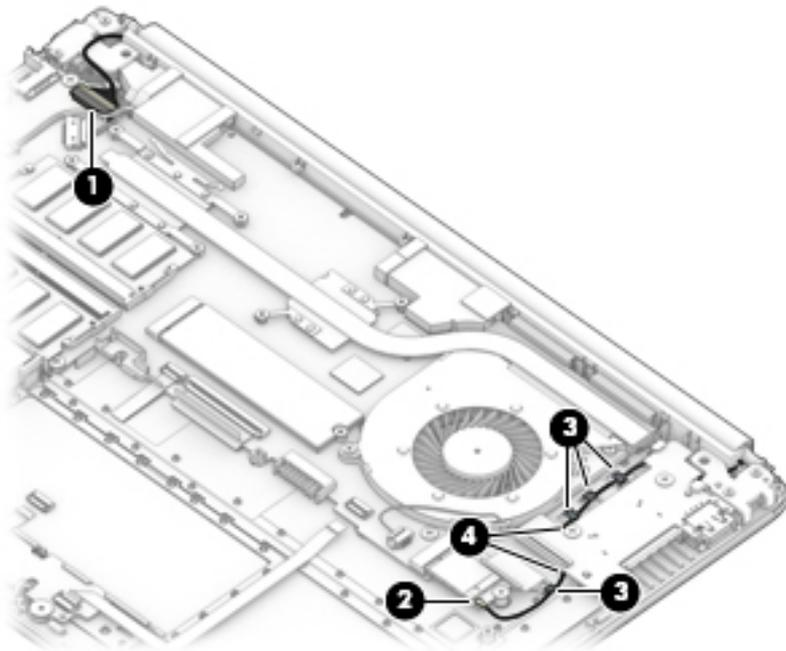
5. Remove the four Phillips M2.5×6.0 screws **(1)** from the display hinges.
