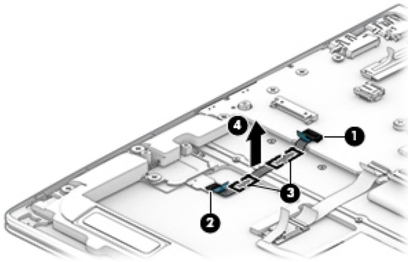
Reverse this procedure to install the fingerprint reader module cable.
