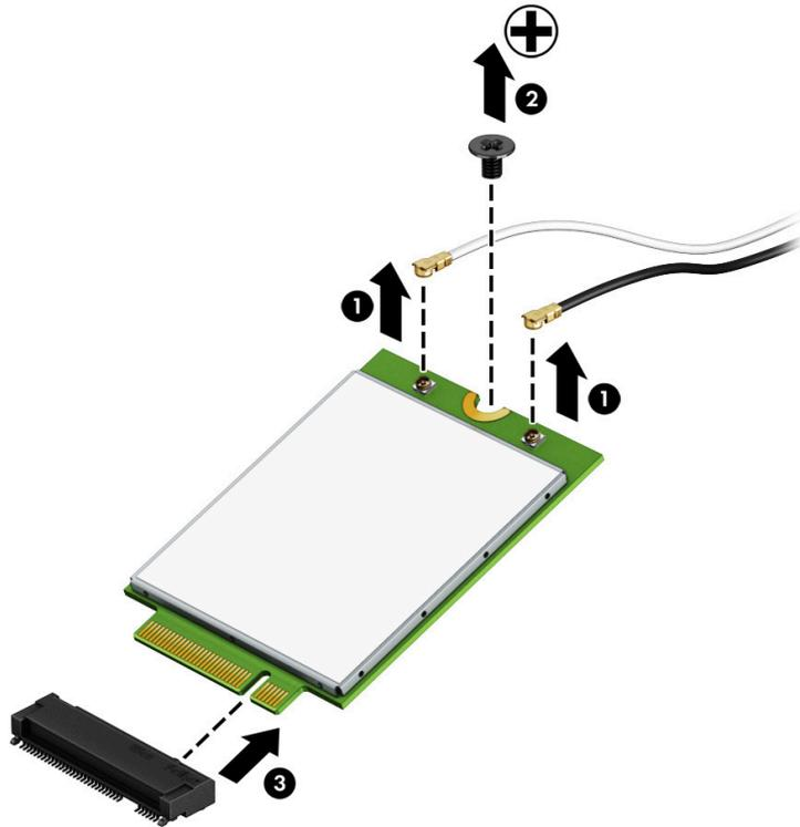
Reverse this procedure to install the WWAN module.
