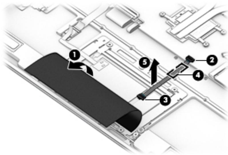
Reverse this procedure to install the TouchPad cable.
