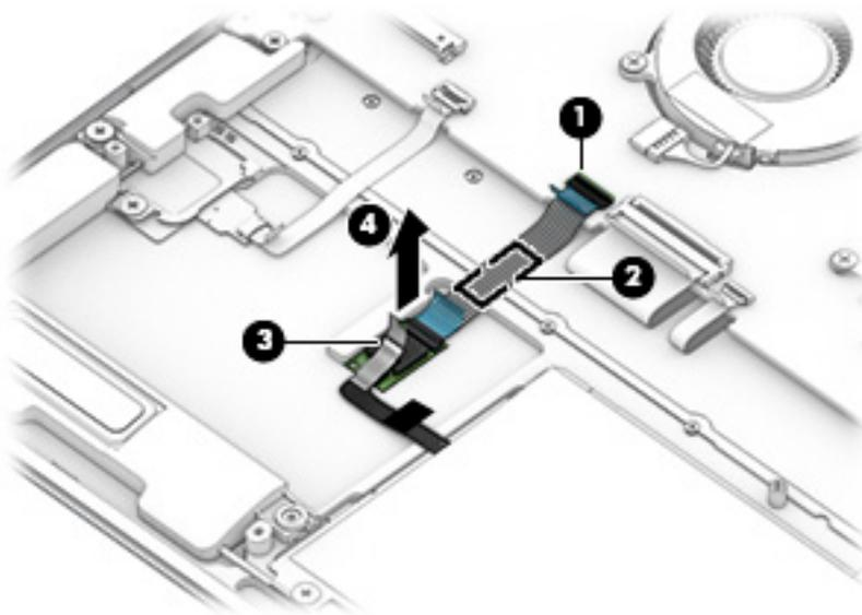
5. Remove the NFC module and cable.
