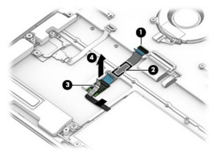
5. Remove the NFC module and cable.
