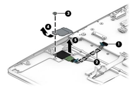
Reverse this procedure to install the fingerprint reader module.
