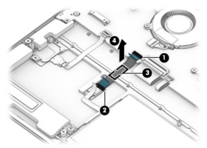
Reverse this procedure to install the NFC module cable.
