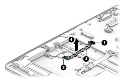
Reverse this procedure to install the fingerprint reader module cable.
