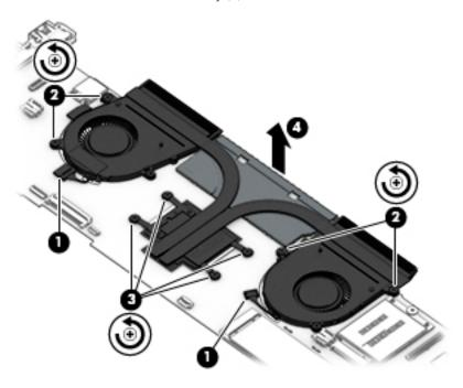
NOTE: The thermal material must be thoroughly cleaned from the surfaces of the fan/heat sink assembly and the system board components each time the fan/heat sink assembly is removed. Replacement thermal material is included with the fan/heat sink assembly and system board spare part kits. Thermal paste is used on the processor (1) and the fan/heat sink assembly section (2) that services it.
