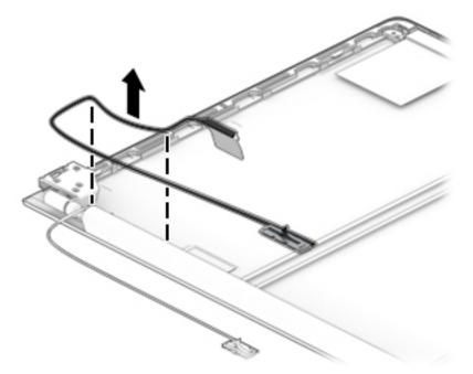
**17.** If it is necessary to replace the camera/ambient light sensor cable:
