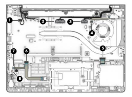
5. Remove the one Phillips M2.0×3.0 screw (1) that secures the USB bracket to the computer, then remove the bracket (2).
