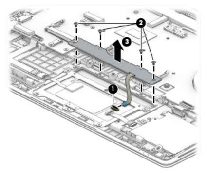
Reverse this procedure to install the TouchPad button board.
