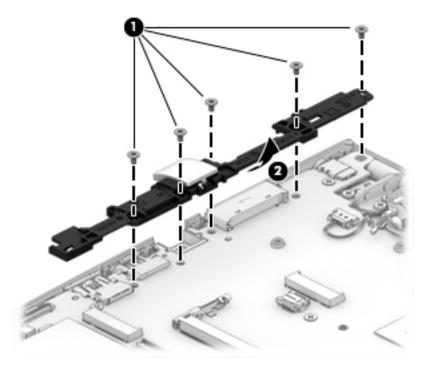
Reverse this procedure to install the RJ-45 assembly.
