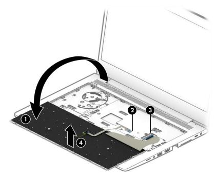
Reverse this procedure to install the keyboard.
