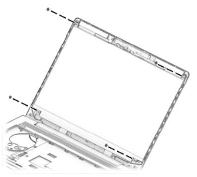
**12.** Rotate the display panel over onto the keyboard **(1)**.
