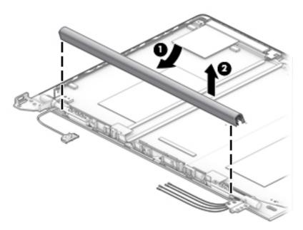
The display hinge cover for non-privacy displays is available in the Hinge Kit for touch displays using spare part number L17975-001. The display hinge cover for non-touch displays is available using spare part number L13683-001.
