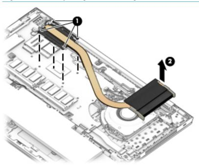
2. Thoroughly clean the thermal material from the surfaces of the system board component (1) and the heat sink (2) each time the heat sink is removed. Replacement thermal material is included with the heat sink and system board spare part kits.
