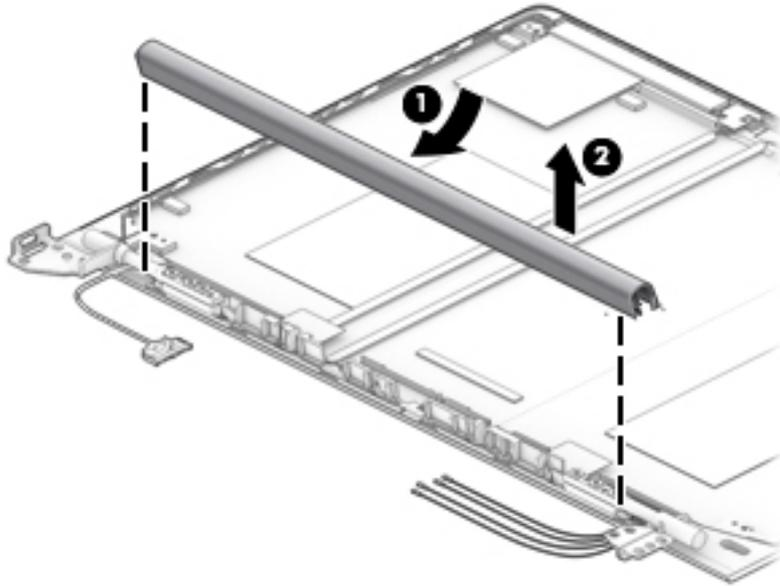
The display hinge cover for non-privacy displays is available in the Hinge Kit for touch displays using spare part number L17975-001. The display hinge cover for non-touch displays is available using spare part number L13683-001.
