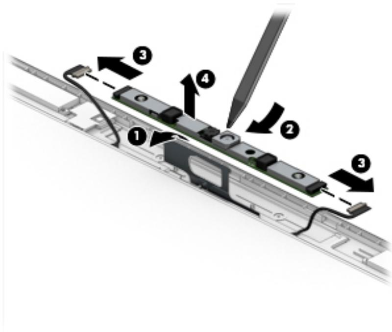
The IR camera module is available using spare part number L13676-001.
