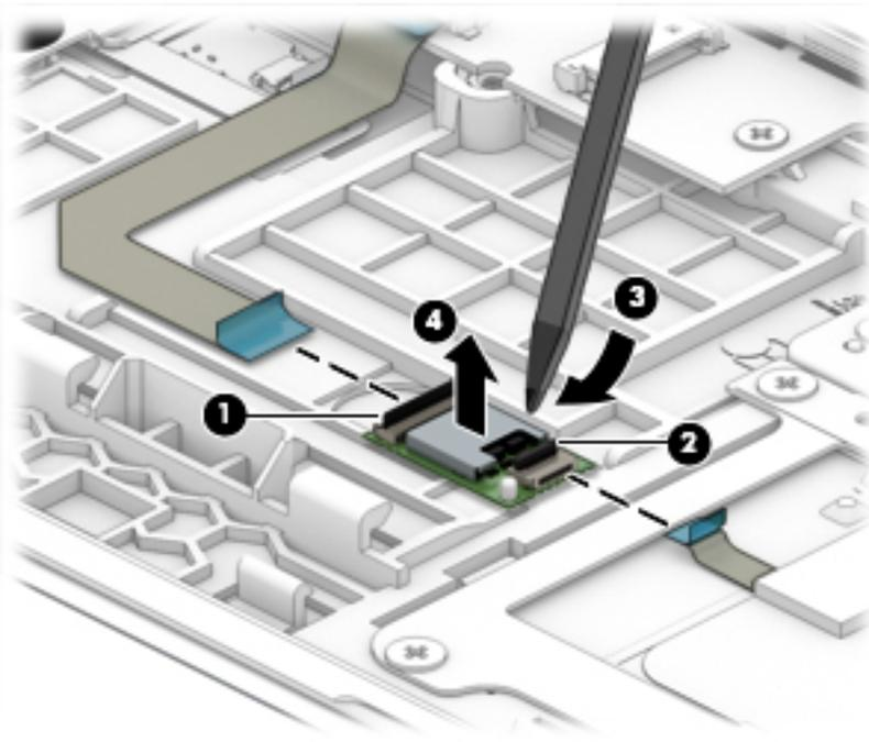
Reverse this procedure to install the NFC module.
