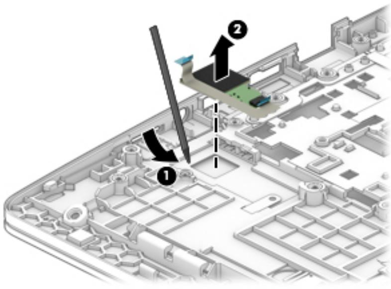
Reverse this procedure to install the fingerprint reader assembly.
