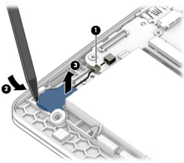
Reverse this procedure to install the RTC battery.
