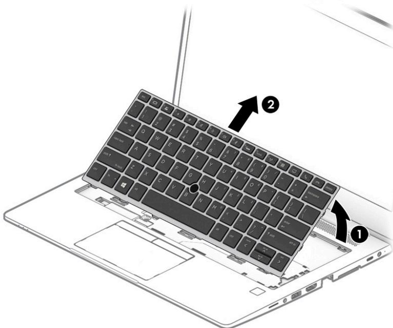
5. With the keyboard resting on the palm rest **(1)**, disconnect the backlight cable from the system board ZIF connector **(2)** (select models only).
