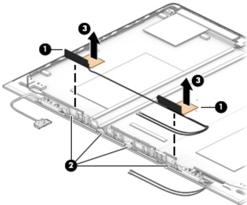
19. If it is necessary to replace the WWAN antenna cables, peel the antennas from the top of the display enclosure (1), remove the antenna cables from the bottom and sides of the display enclosure (2), and then remove the antenna cables (3).
