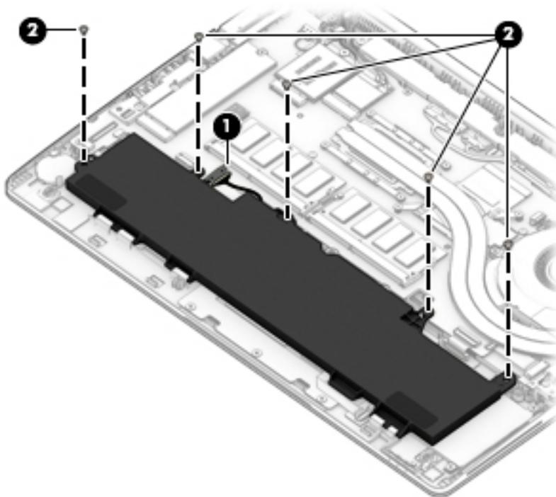
3. Rotate the top of the battery upward **(1)**, and then lift the battery out of the computer **(2)**.
