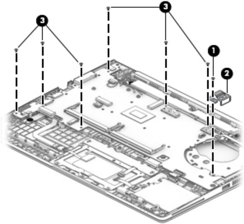
7. Lift the right side of the system board up at an angle **(1)**.
