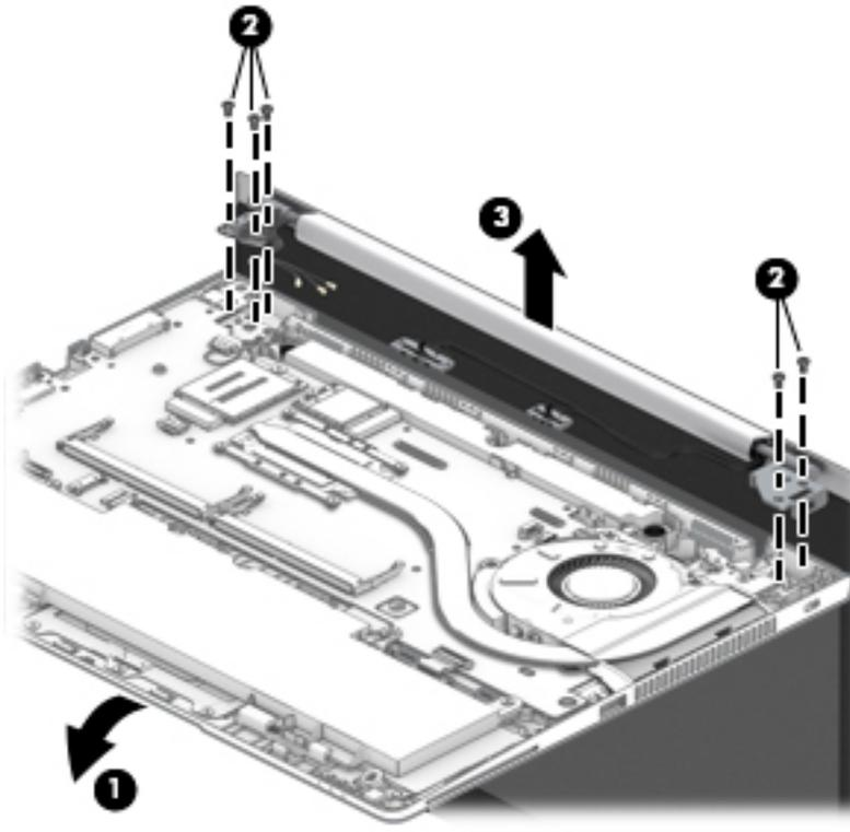
6. To remove the display bezel, first rotate top of hinge cover away from display enclosure to disengage the tabs **(1)**, and then pull the cover off the enclosure **(2)**.
