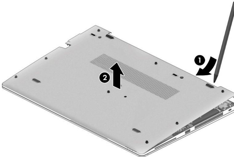
Reverse the removal procedures to install the bottom cover.
