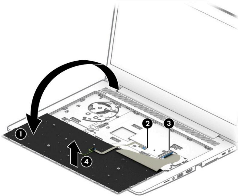
Reverse this procedure to install the keyboard.
