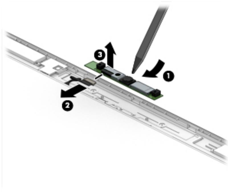
The HD camera module is available using spare part number L13677-001. The microphone module is available using spare part number L13689-001.
