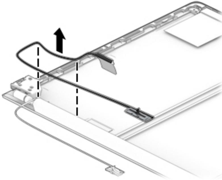
17. If it is necessary to replace the camera/ambient light sensor cable:
