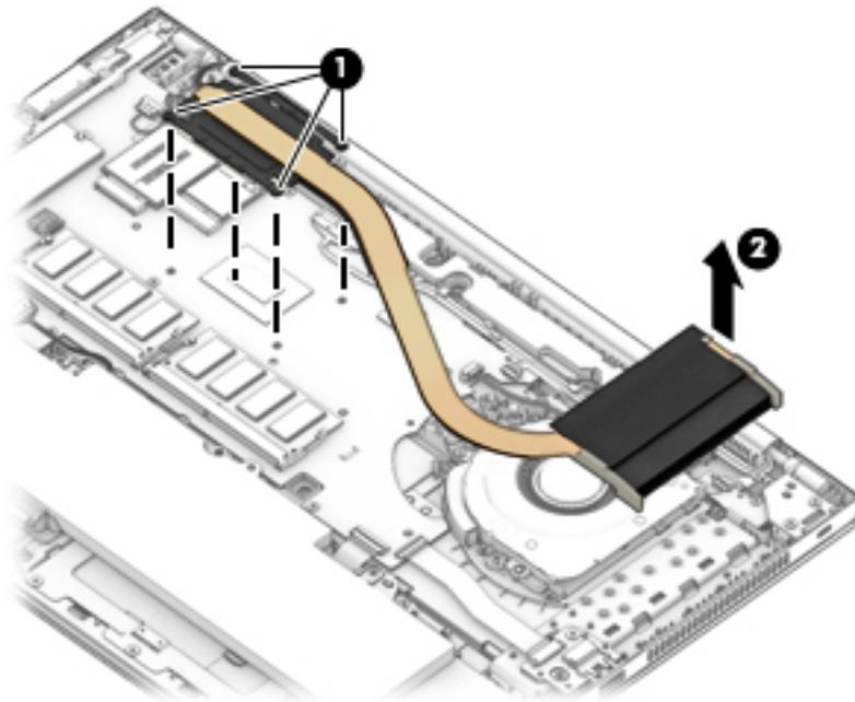
2. Thoroughly clean the thermal material from the surfaces of the system board component **(1)** and the heat sink **(2)** each time the heat sink is removed. Replacement thermal material is included with the heat sink and system board spare part kits.
