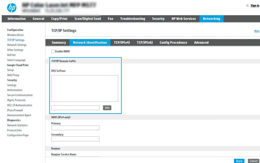
The screenshot shows the HP EWS interface for TCP/IP Settings. The 'Networking' tab is selected, and the 'Network Identification' sub-tab is active. A red box highlights the 'TCP/IP Domain Suffix' section, which includes a 'DNS Suffixes' list and an 'Add' button. Below this, the 'WINS (IPv4 only)' section has 'Primary' and 'Secondary' input fields. The 'Bonjour' section has a 'Bonjour Service Name' input field. 'Apply' and 'Cancel' buttons are at the bottom right.
