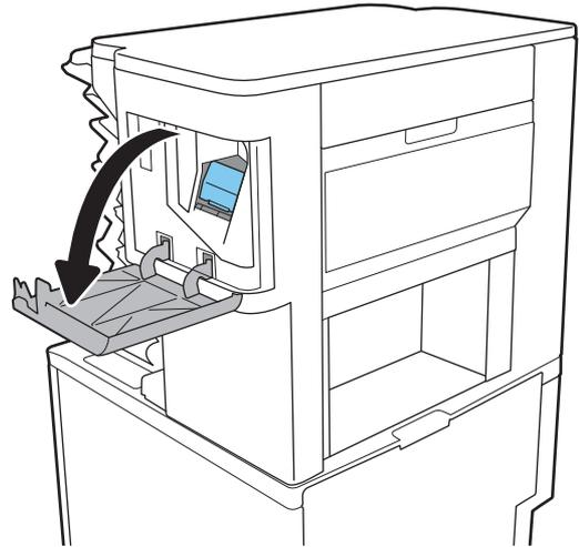
2. Pull down the colored handle on the staple carriage, and then pull the staple carriage straight out.
