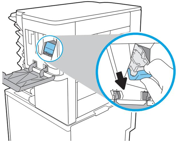
3. Lift up on the small lever at the back of the staple cartridge.
