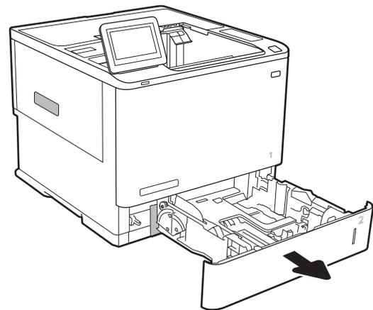
2. Adjust the paper-length and paper-width guides by squeezing the blue adjustment latches and sliding the guides to the size of the paper being used.
