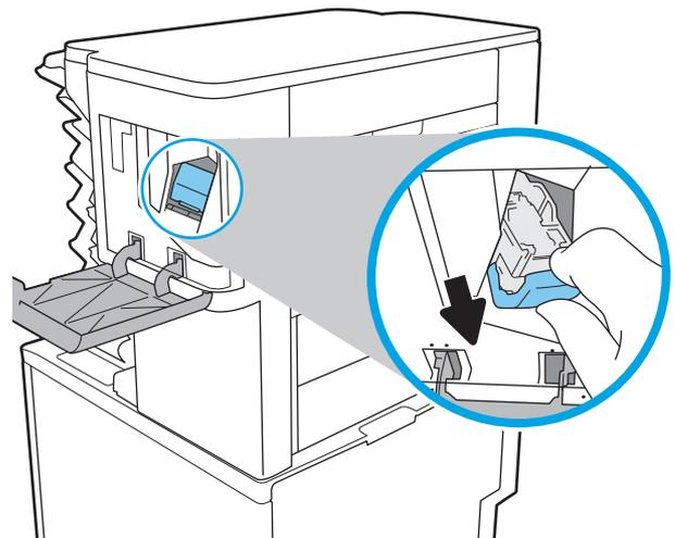
3. Lift up the empty staple cartridge to remove it from the staple carriage.
