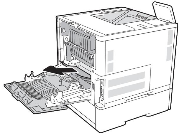
3. Remove the fuser by grasping the two side latches and pulling the fuser straight out of the printer.
