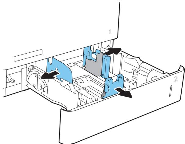
3. Load paper into the tray. Check the paper to verify that the guides touch the stack, but do not bend it. For information about how to orient the paper, see [Table 2-2 Tray 2 and the 550-sheet trays paper orientation on page 25](#).
