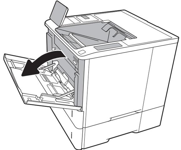
2. Adjust the paper-width guides by squeezing the blue adjustment latch and sliding the guides to the size of the paper being used.
