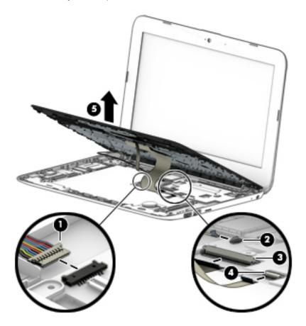
Reverse this procedure to install the keyboard/top cover.
