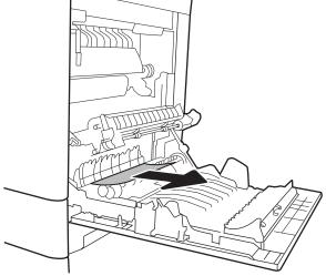
3. If paper is visible entering the bottom of the fuser, gently pull downward to remove it.
