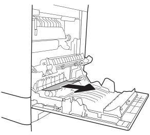
**10.** If paper is visible entering the bottom of the fuser, gently pull downward to remove it.
