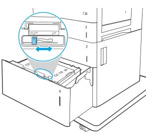
3. Rotate the paper-stop lever to the correct position for the paper being used.
