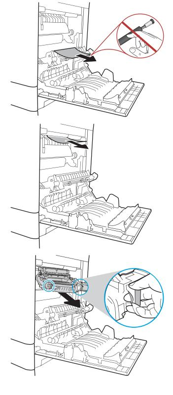
Open the jam-access door on the fuser. If paper is jammed inside the fuser, gently pull it straight up to remove it. If the paper tears, remove all paper fragments.
