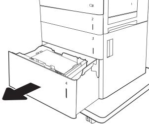
2. Remove any jammed or damaged sheets of paper. Verify that the tray is not overfilled and that the paper guides are adjusted correctly.
