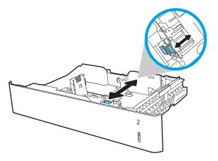
3. Adjust the paper-length guide by squeezing the adjustment latch and sliding the guide to the size of the paper being used.
