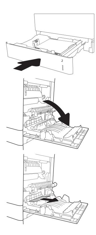
7. If paper is visible entering the bottom of the fuser, gently pull downward to remove it.
