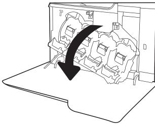
3. Grasp the handle of the used toner cartridge and pull out to remove it.
