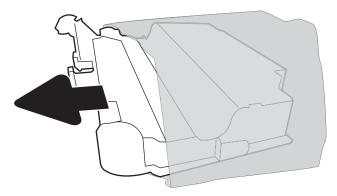
**6.** Install the new unit into the printer. Make sure the toner-collection unit is firmly in place.
