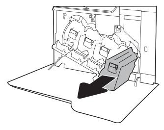
4. Remove the new toner cartridge from its packaging by removing the plastic end caps, removing the cartridge from the plastic bag, and then removing the orange protective shield. Save all packaging for recycling the used toner cartridge.
