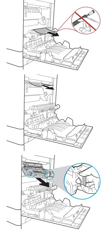
10. Open the jam-access door on the fuser. If paper is jammed inside the fuser, gently pull it straight up to remove it. If the paper tears, remove all paper fragments.
