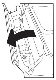
Grasp the top of the toner-collection unit and remove it from the printer.
