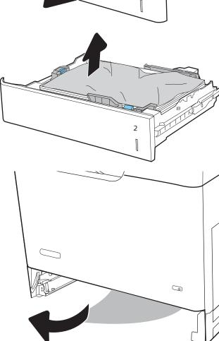
3. Gently remove any paper from the feed rollers inside the printer. First pull the paper to the left to release it, and then pull it forward to remove it.
