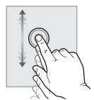
Touch the screen and then move your finger vertically to scroll the screen up and down. When scrolling through menus, briefly touch the screen to stop the scrolling.
